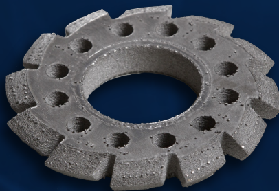
VBN 3D prints part in near-net-shape (hardened)
