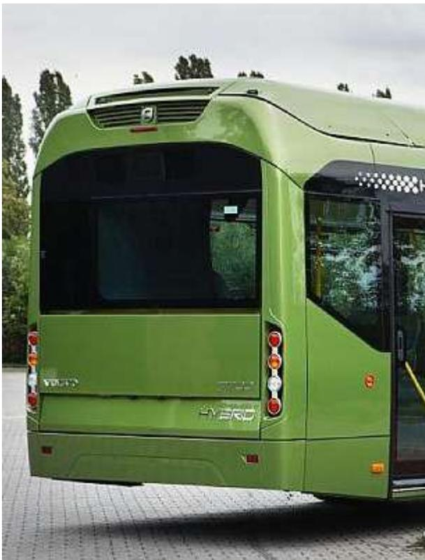
**Test production of a city bus rear end using 3Dlitecomp technology**
