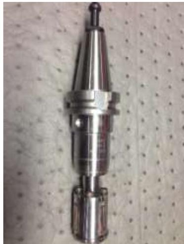
*Fig 3. ANS Triboconditioning of Volvo rocker arm in standard machine with prototype tool head*
