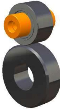
*Fig 2. Pin/roller contact in test rig at Halmstad University*
