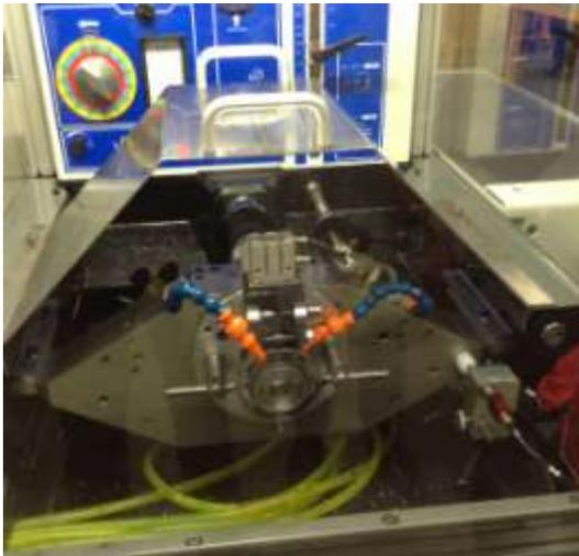
*Fig 1. Treatment of Volvo cam follower rollers in Alvesta*
