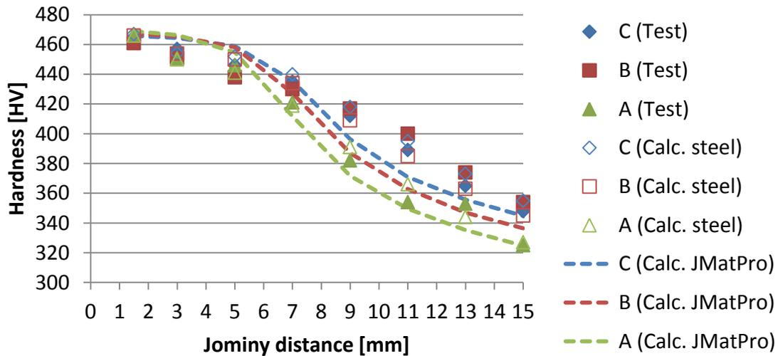
**Figure 16 Hardenability of the three heats of 16NiCrS4 used in this project. Heats are named A, B and C. Hardenability is given as: (Test): Jominy test according to ISO 642; (Calc. steel): Calculated with model from steel supplier; (Calc. JMatPro): Calculated with generic model built in to JMatPro software (version 8).**
