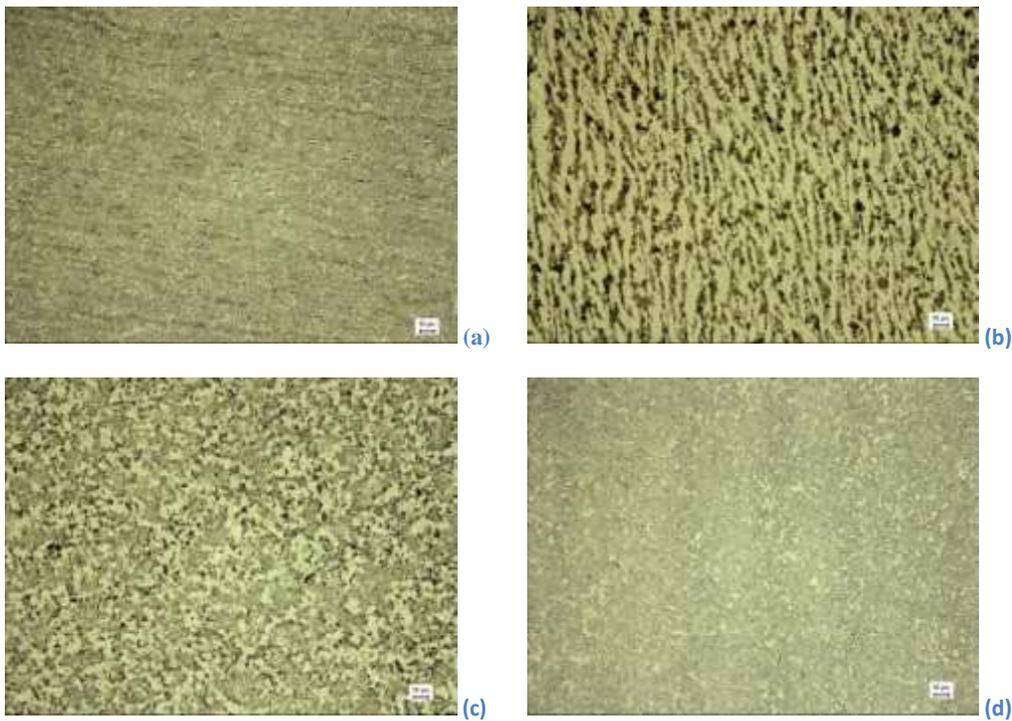
Figure 8 Representative microstructure of parts and materials used in cutting tests. (a) The planet gear of Volvo, (b) the 2nd gear of Scania, (c) used bar of Ovako 157C and (d) used bar of Uddeholm Orvar Supreme.
