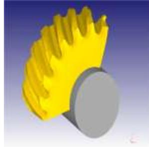
Simulation of penetration of 6 mm of tool into blank.
