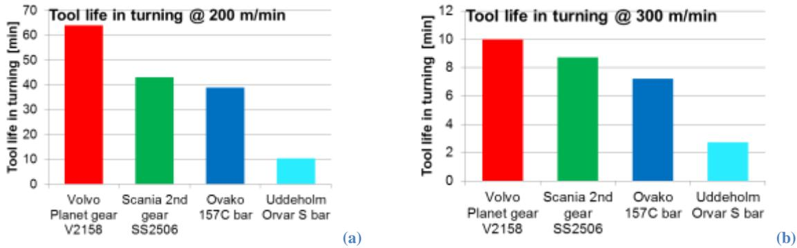
Figure 9 Tool life of the tested materials and geometries of the project at (a) 200 m/min and (b) 300 m/min.
