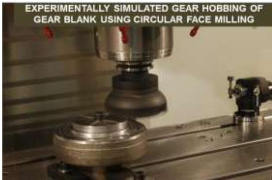
Figure 12 The machining test designed to mimic the conditions of conventional gear hobbing.
