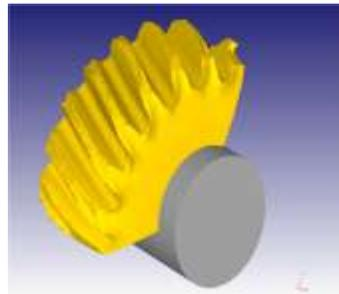
Simulation of full penetration of 13 mm of tool into blank.
