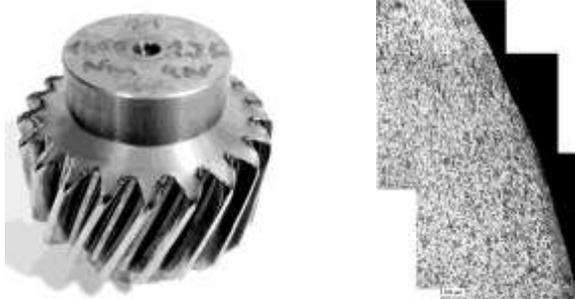
Figure 5 Gear rolled gear wheel. Figure 6 Etched cross section of flank area.
