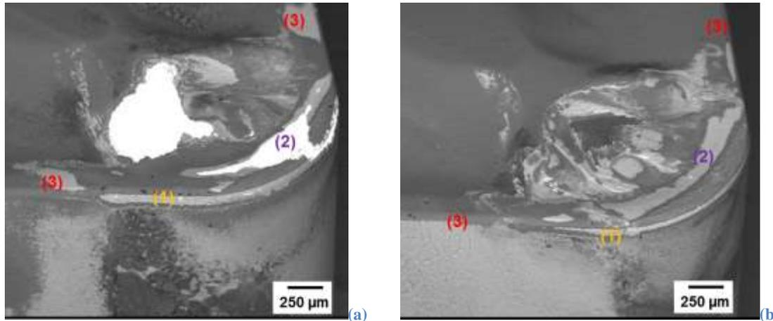
Figure 14 Micrographs of the cutting inserts used in field tests at Swepart Transmission. 404 planet gears were rough turned with (a) Scania SS2506 steel and (b) Ovako 158Q steel. (SEM-BS of etched cutting inserts)
