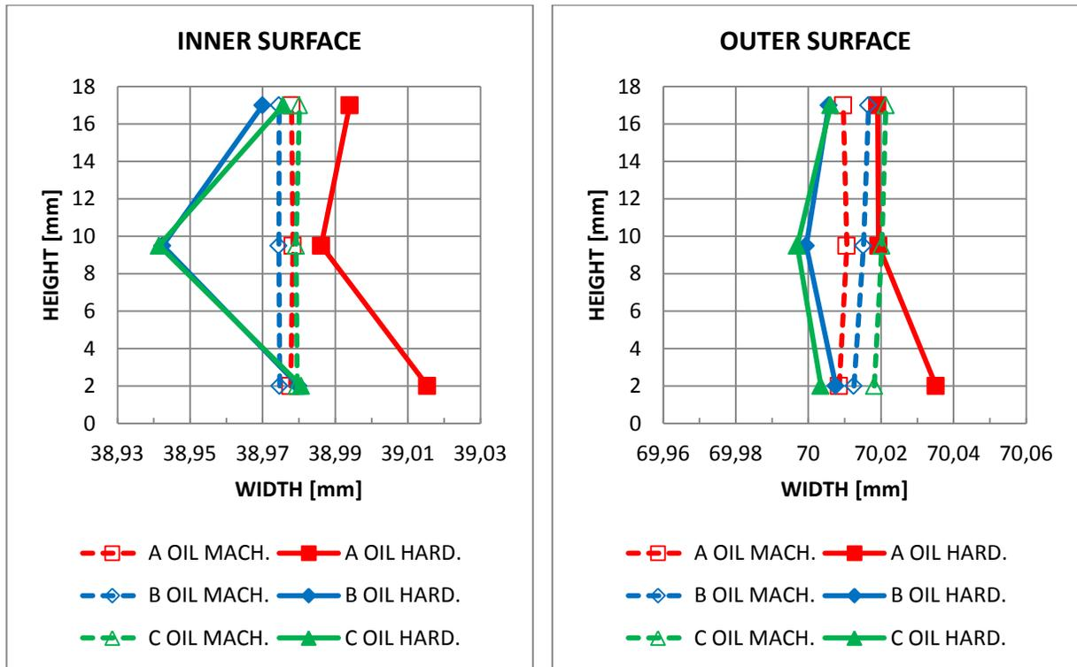
Figure 17 Radial distortion of oil quenched rings. The inner and outer surfaces becomes convex and concave, respectively. The inner diameter shrinks for heats B and C, but grows for heat A.
