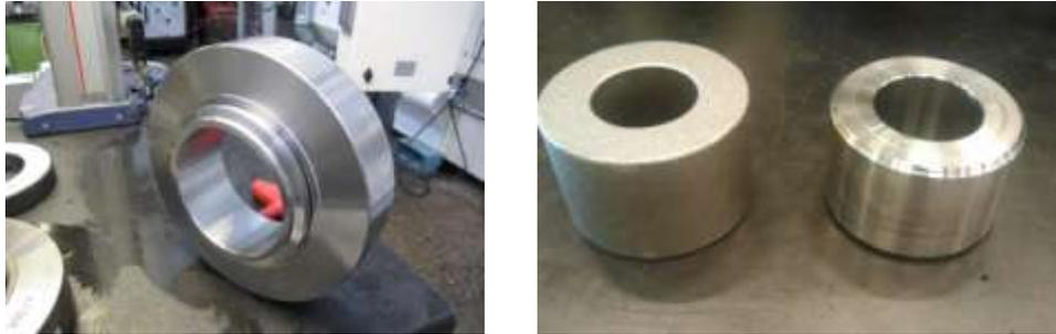
Figure 7 The 2nd gear of Scania and the planet gear of Volvo.
