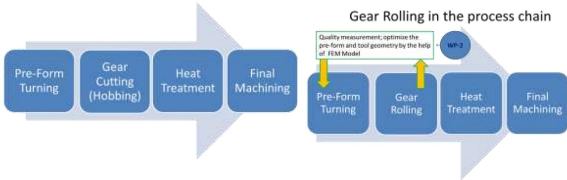
Figure 2 Conventional production chain for gear wheels. Figure 3 Production chain with gear rolling.
