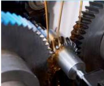
Figure 1 Gear rolling.
