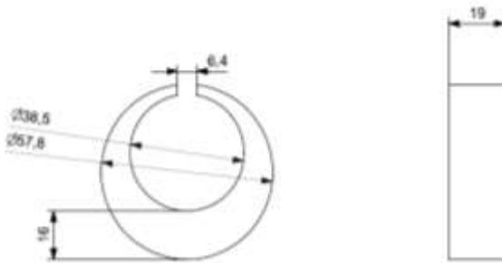
Figure 15 Shape of C-ring used for heat treatment experiments, measurements are given in [mm].
