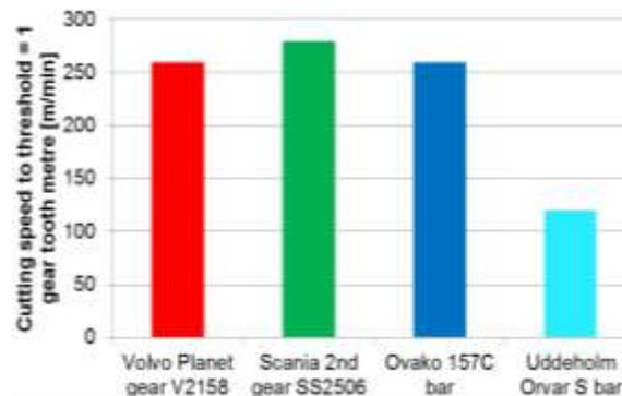
Figure 13 Bar chart of transition speed to meet the criterion of go and no-go of removed chip volume that corresponds to one gear root metre.
