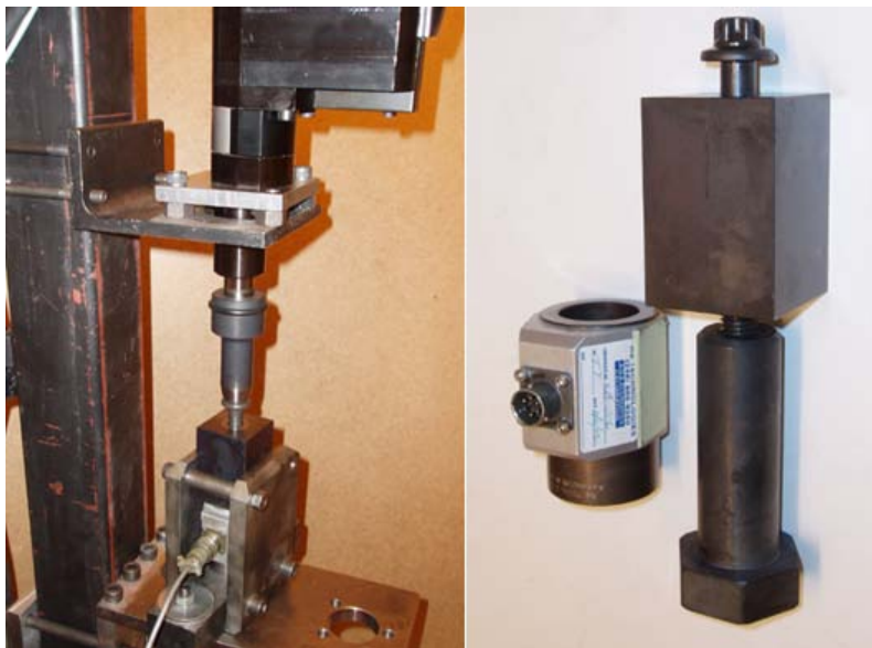
Figure 3. Atlas Copco's test rig for the development of ultrasonic assembly.
