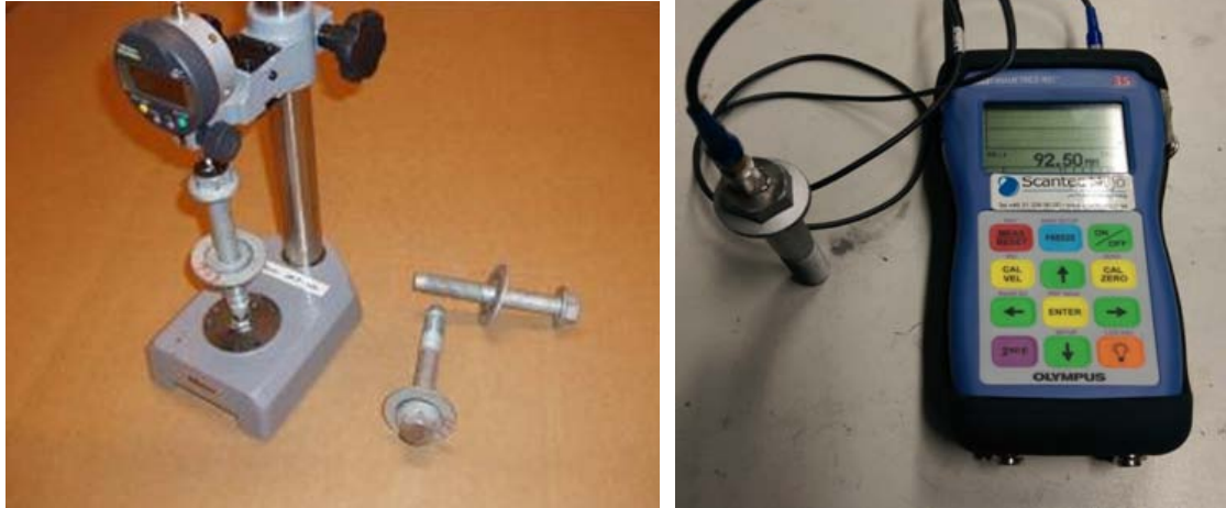
Figure 5. Equipment for mechanical length measurement (left) and ultrasound (right).
