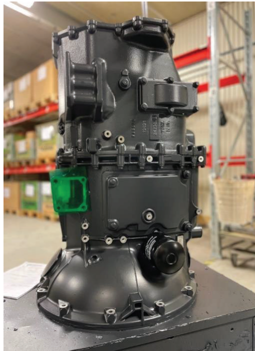
Figure: A remanufactured Scania gearbox
