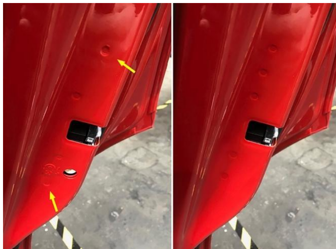
Figure 1. Spot weld position without (left) & with (right) perceived quality consideration
