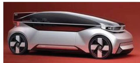
Volvo Cars 360c concept car: all-electric, fully autonomous, modular vehicle
