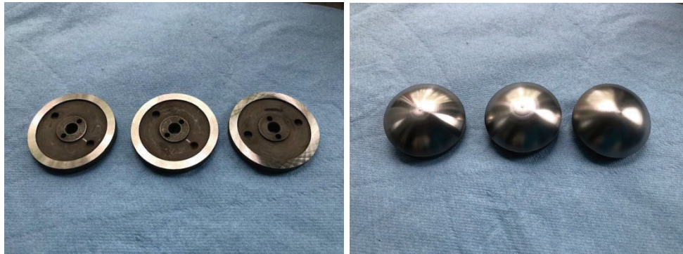
Figure 8. From left to right, circumferential rough, circumferential smooth, crosshatched surface and the pins used during the tribotest.
