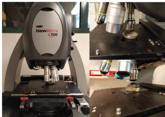
Figure 5. The optical profiler tool used to scan all surfaces (left), the disc positioned for measuring (top right), the pin fixture to facilitate orientation (bottom right).
