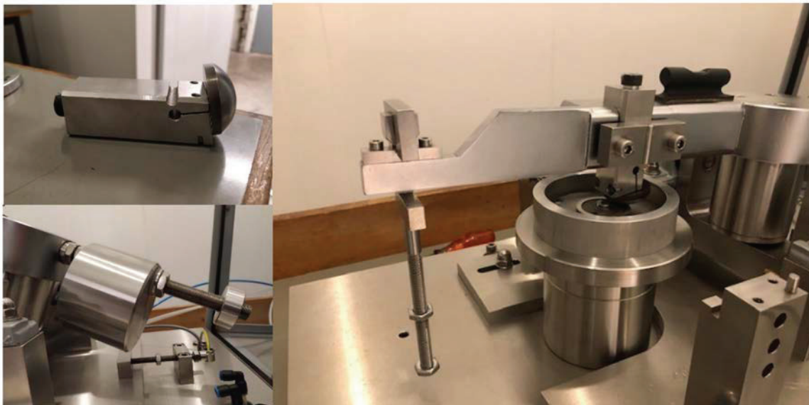
Figure 9. The pin-on-disk tribotesting machine setup.
