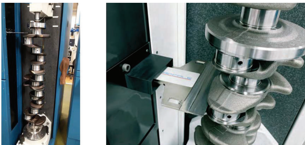
Figure 2. Adcole CCMM. Left: Image of the actual machine at dept. BE63730. Right: Image from Adcole homepage.
