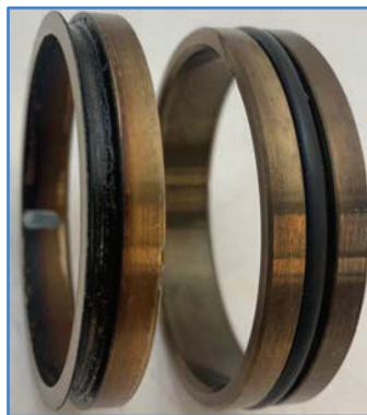
Figure 22. Left: Wear NOK (O-ring removed), Right: Wear OK .
