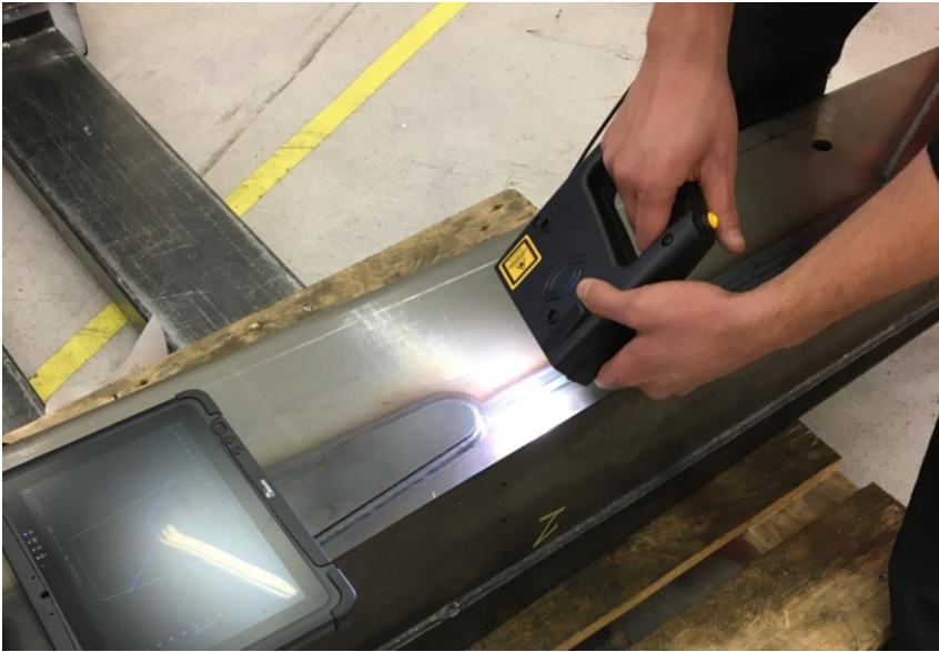
Figure 9. Winteria Flex hand-held system measuring an a5 fillet weld.
