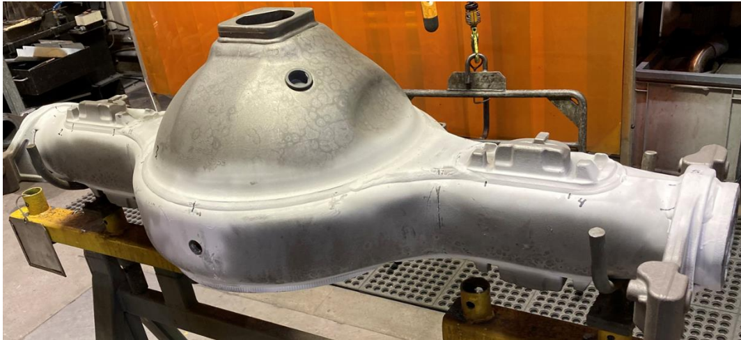
Figure 17. The Scania type of rear axle used in test with laser scanning.
