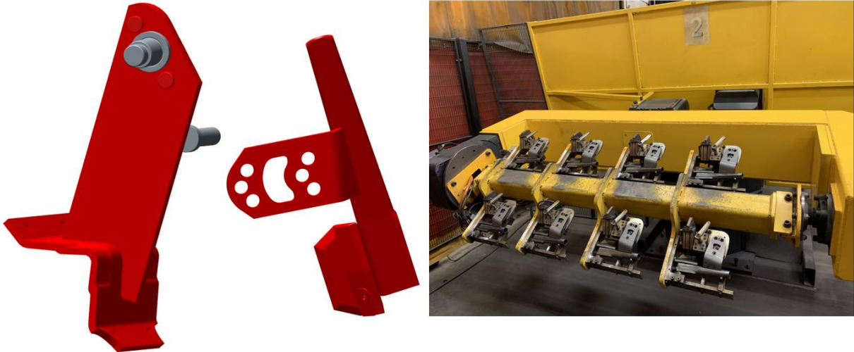
Figure 15. Welded high-volume part for a combine harvester (left) and one side of the positioner with the parts mounted in the welding fixture (right).
