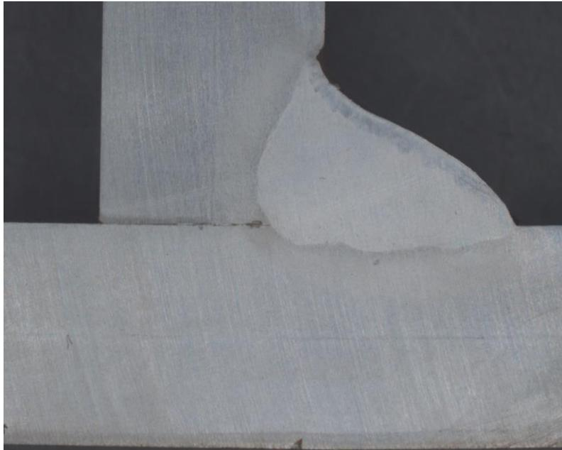
*Figure 16 Cross-section of verification run ID 103, weld with minimized Cold laps, however with an undercut present in upper weld toe (upper toe not included in the model).*
