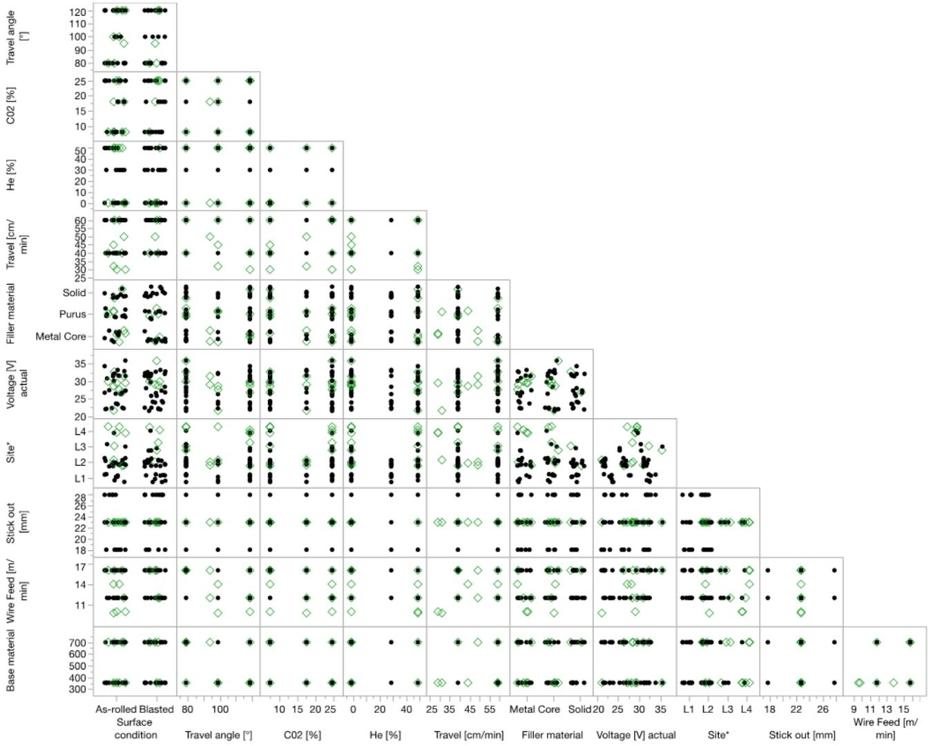
Figure 13 Factors and factor levels for the 36 run experimental design represented by black dots, and the 16 run Augmented design represented by Green diamonds.
