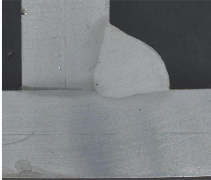
*Figure 17 Cross-section of verification weld, run ID 102, with Cold laps maximized.*
