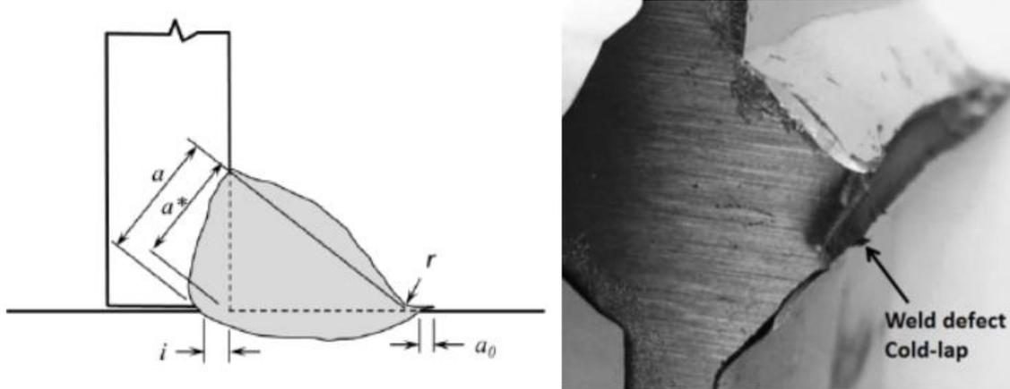
Figure 1 ) a) Fillet weld geometrical features which are influencing the fatigue strength;  $a_0$ ... cold lap depth [Source: supplement to ISO 5817] b) Fatigue tested welded specimen with cold laps indicated [Swerea KIMAB project, from 2016].
