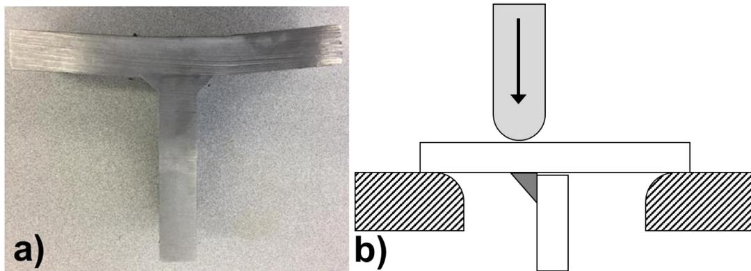
*Figure 5 Bend testing: a) illustrates a slightly bent sample after bend testing. b) Schematic view of the bend-testing method. Note the tool positioning just above the weld toe.*
