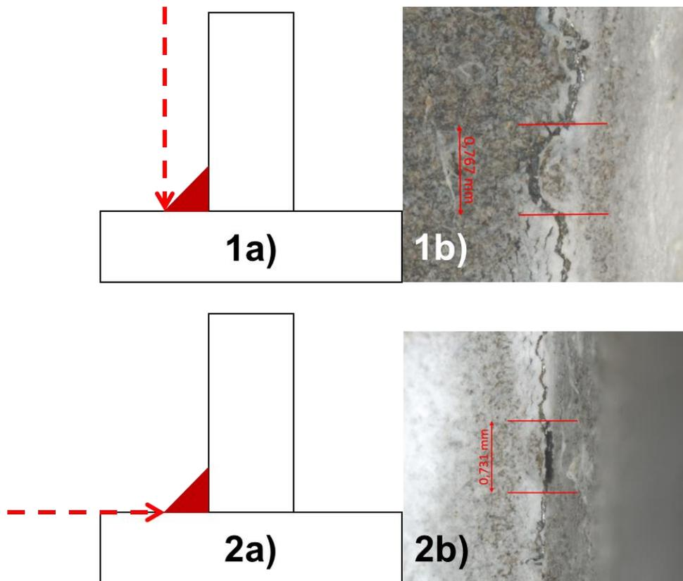
Figure 6 1a) Schematic view of LOM image obtained along the Vertical plate. 1b) Example of LOM image obtained in Vertical view. 2a) Schematic view of LOM image obtained along the Horizontal plate. 2b) Example of LOM image obtained in horizontal view.
