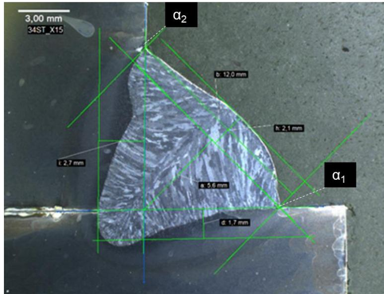
Figure 3 Example of measurements by cross section and LOM. Measured in LOM were: Throat thickness (a), Weld penetration (i), Weld side penetration (d), Weld reinforcement (h), weld bead width (b) and Weld toe angles ( $\alpha_1$  &  $\alpha_2$ )
