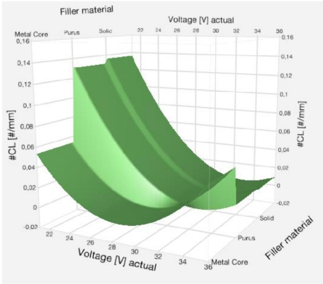
Figure 18 Response surface for Number of Cold laps per tested mm [#CL/mm], Filler material and Voltage actual (Measured Voltage).
