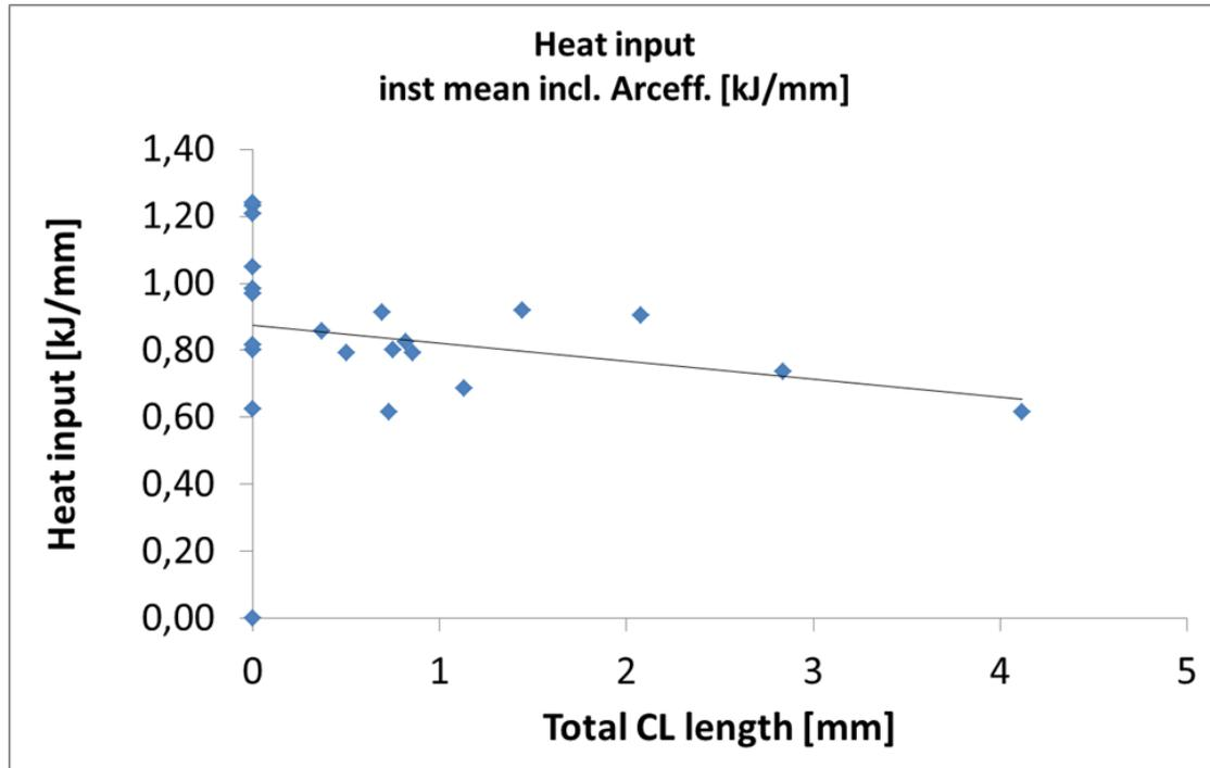
Figure 11 Results from PREMOD samples, influence of Heat input [kJ/mm] on the sum of measured Cold laps [mm]. Heat input above 1.0 kJ/mm results in zero Cold laps found
