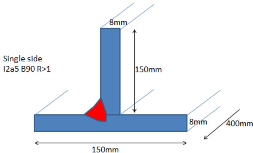
*Figure 8 Schematic view of welded samples gathered from the participating companies for the classical testing.*
