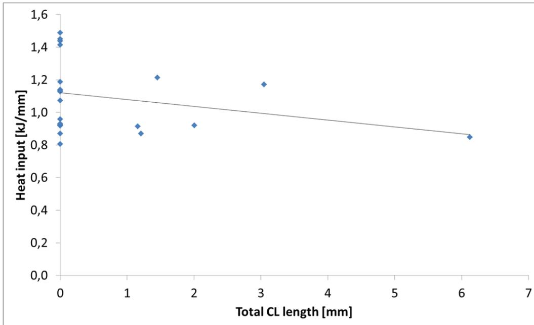
Figure 10 Results from classical trials, influence of Heat input [kJ/mm] on the sum of measured Cold laps [mm]. Heat input above 1.3 kJ/mm results in zero Cold laps found
