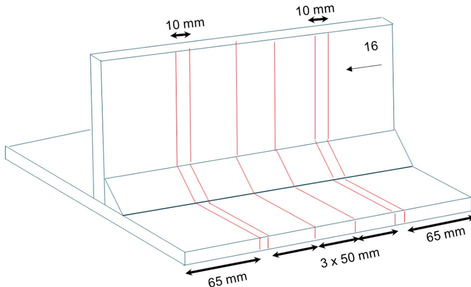
*Figure 2 Illustration of how welded samples were cut into smaller samples before evaluation, ID-number and welding direction is marked in upper right corner.*
