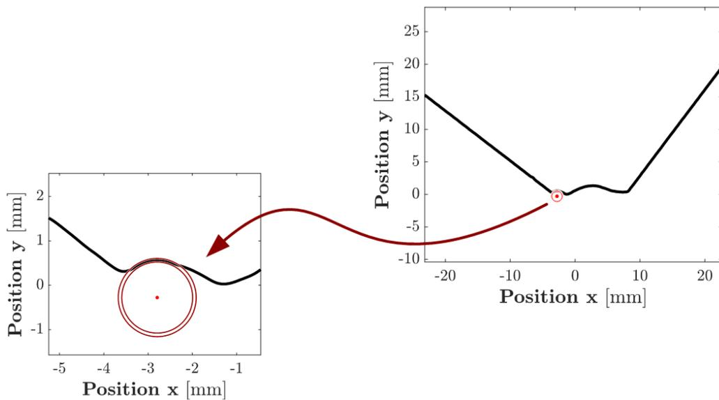
*Figure 7 Illustration of radius fit algorithm for detection of Cold laps.*
