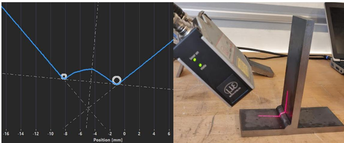
Figure 4 Image of the laser scan process (right) and schematic view of the weld profile obtained (left).
