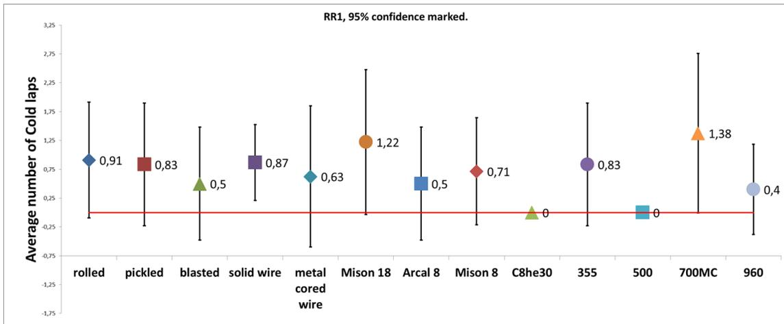
Figure 9 Results from classical testing, Average number of Cold laps per welding condition and 95% confidence interval marked.
