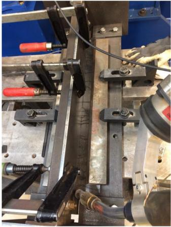
Figure 3. Fixture used in the welding trials.
