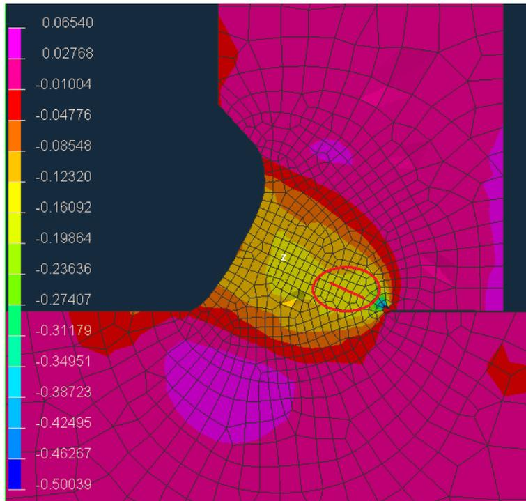
Figure 30. Strain distribution in specimen welded with half V-joint and 0mm gap. Area of interest marked in red circle.
