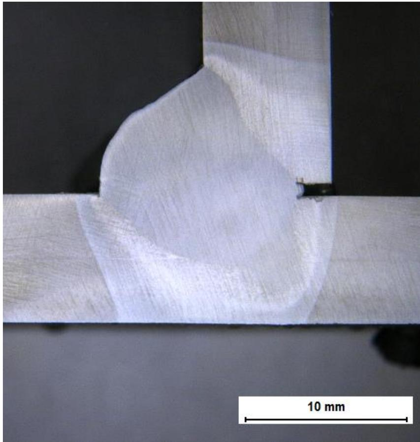
*Figure 15. Cross-section of weld used for 2D-simulations.*
