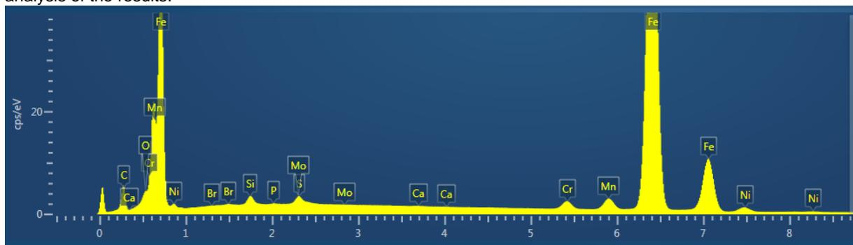
*Figure 13, EDS analysis of the elements on the crack surface.*
