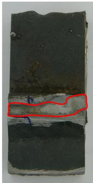
Figure 11, A hot crack that has been broken open, the crack is marked with the red line
