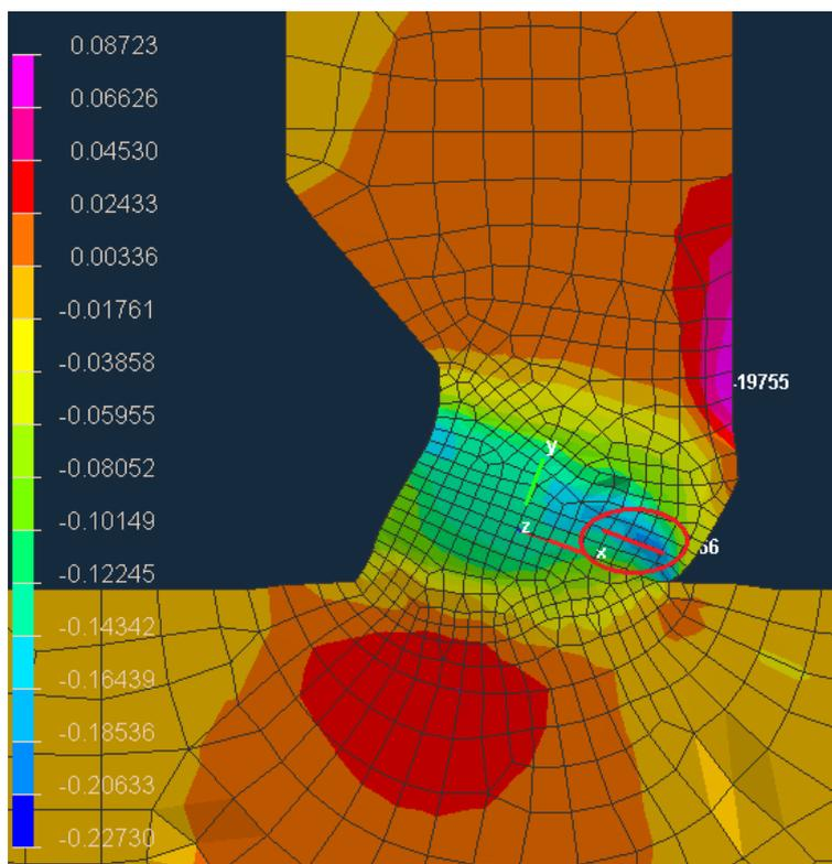
Figure 31. Strain distribution in specimen welded with half V-joint and 2,5mm gap. Area of interest marked in red circle.
