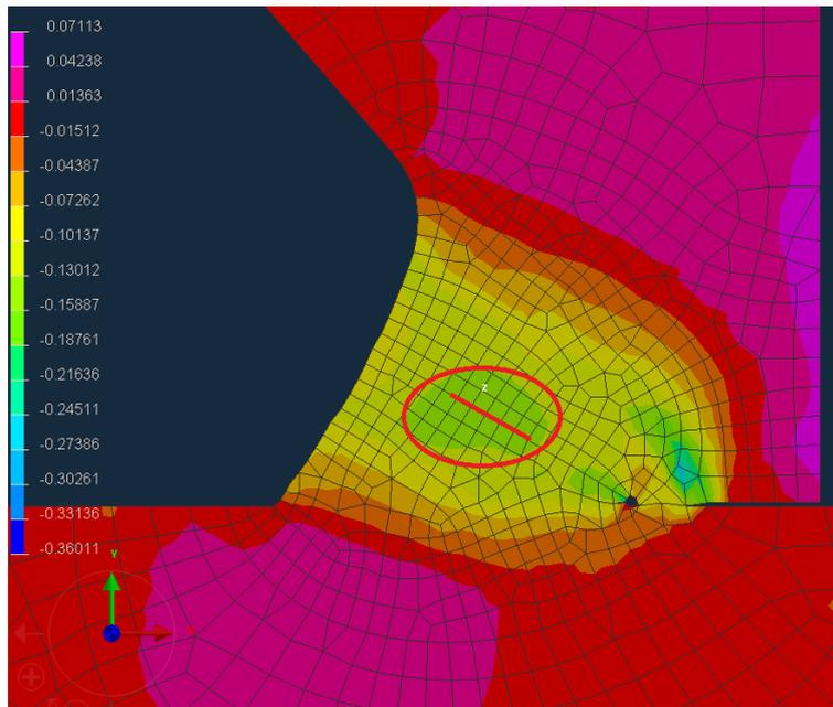
Figure 34. Strain distribution in specimen welded with half V-joint with land and 0mm gap. Area of interest marked in red circle.
