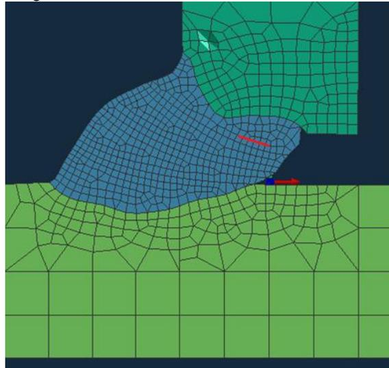
*Figure 19. Image showing the mesh of the specimen from the first part of the 3D-simulations, specimen welded with low aim of the torch.*
