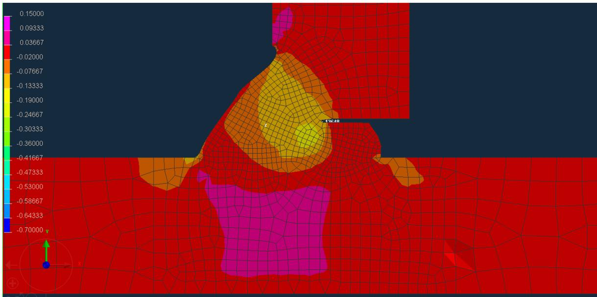
Figure 22. Strain distribution for case with high aim.
