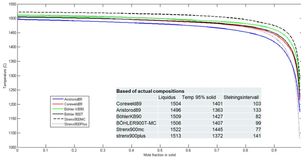
Figure 10 Solidification range for all base and filler materials used in this study
