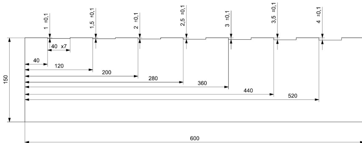
Figure 2. Illustration of milled grooves in the web plate.
