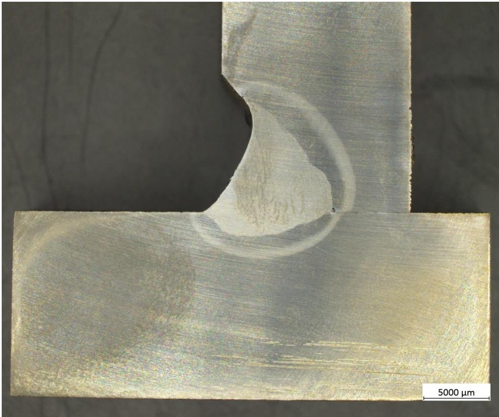
*Figure 26. Specimen welded at Huddig, half V-joint and 0mm gap.*
