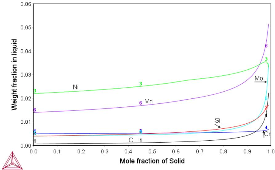
Figure 8 Segregation of alloying elements in a typical filler material used in this study
