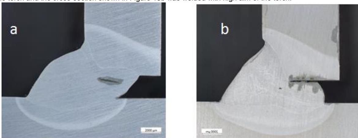
Figure 18. Cross-sections of welds for 3D-simulations. The welds are produced with the same base- and filler material. Specimen (a) is welded with low aim of the torch and specimen (b) is welded with high aim of the torch.
