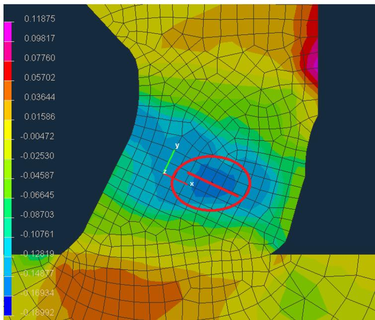
Figure 35. Strain distribution in specimen welded with half V-joint with land and 2,5mm gap. Area of interest marked in red circle.
