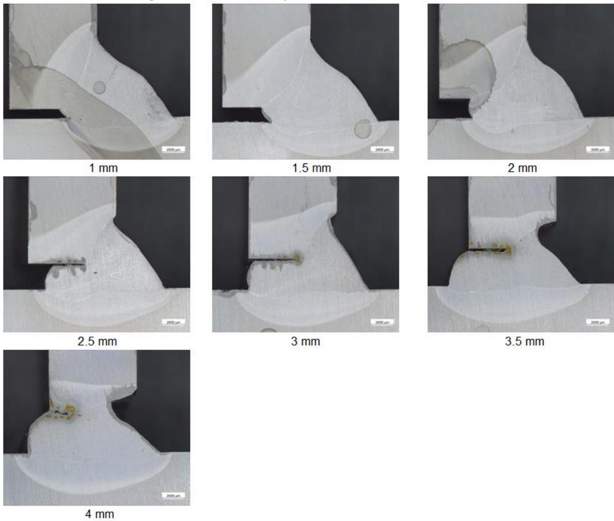
*Figure 6. Cross-sections from series welded with high aim.*
