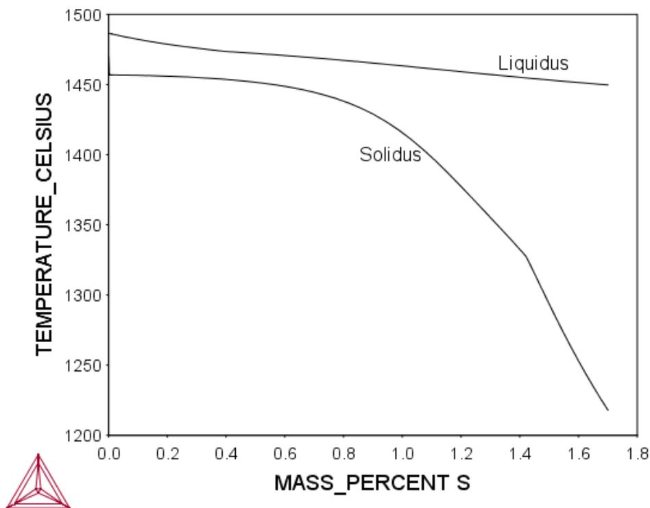
Figure 7: Equilibrium calculation of liquidus and solidus lines for a fictive C-Mn steel composition as a function of Sulphur content in the steel.
