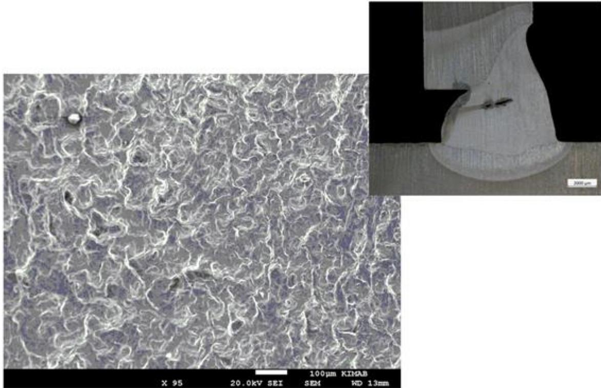
*Figure 12, SEM analyzed surface of the crack in weld 63.*
