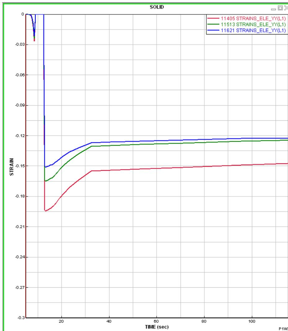
Figure 24. Continuous strain for elements in area most prone to form hot cracks for specimen welded with high aim.
