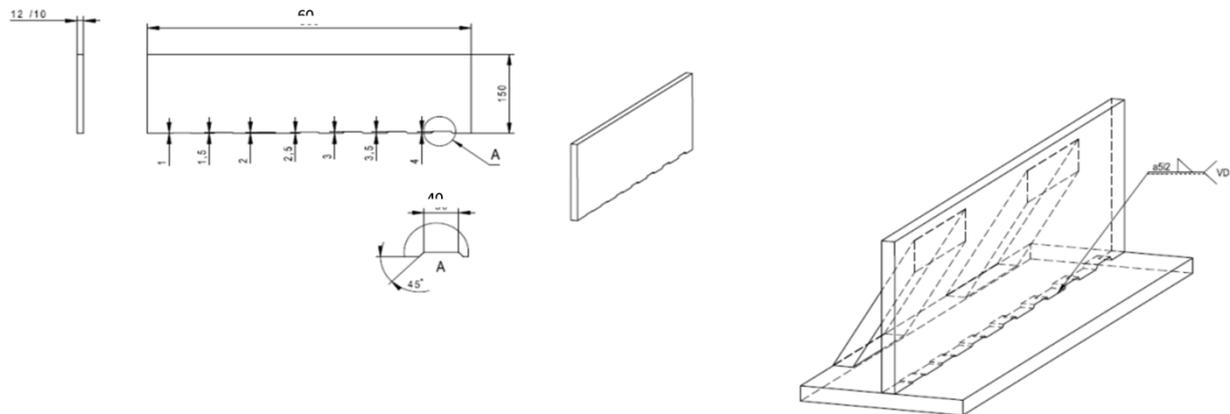
Figure 1. Schematic illustration of the experimental set-up from the trials at Volvo.
