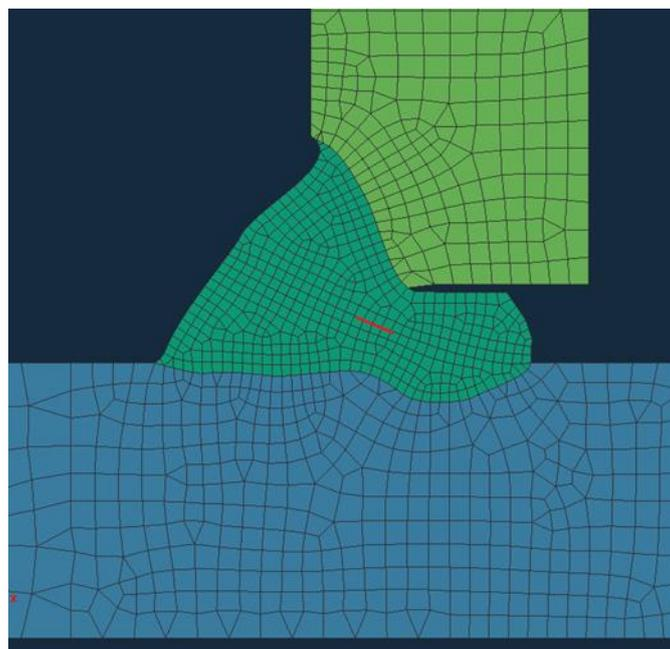
*Figure 20. Image showing the mesh of the specimen from the first part of the 3D-simulations, specimen welded with high aim of the torch.*
