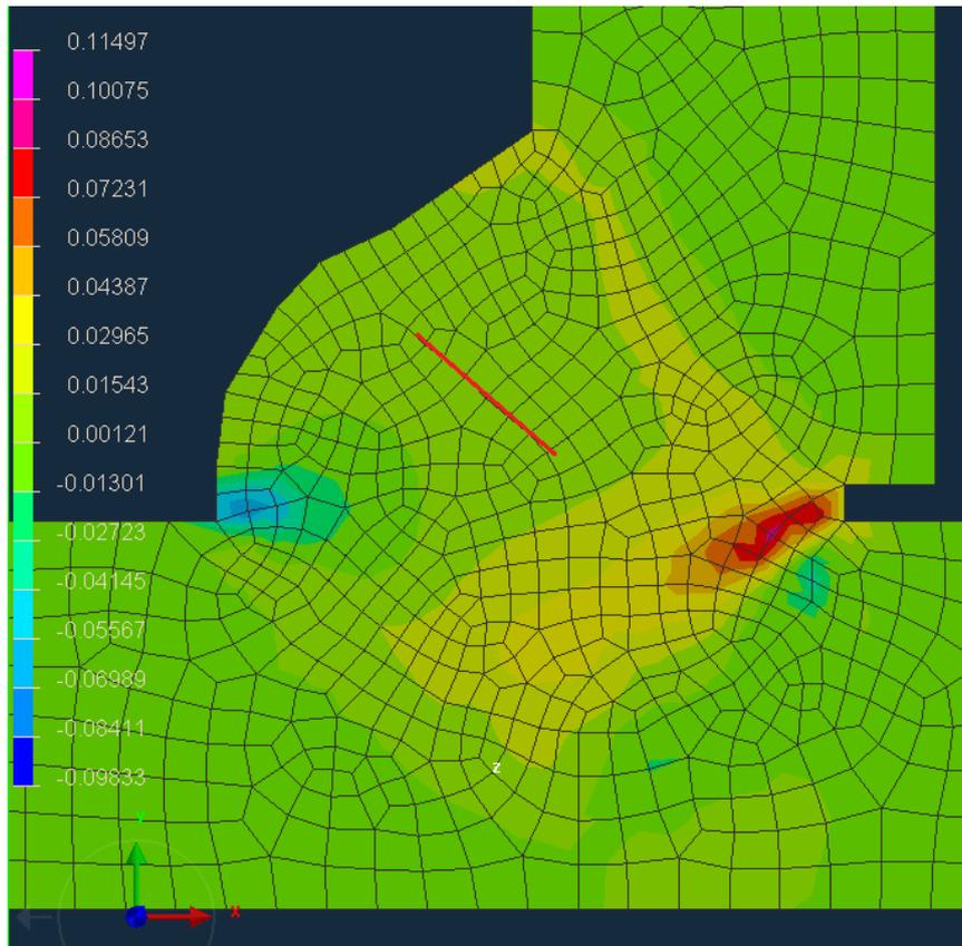
Figure 17. Strain distribution from 2D-simulations.
