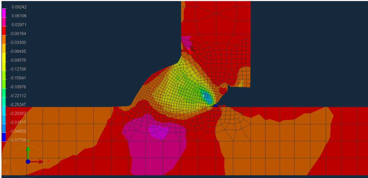
Figure 21. Strain distribution for case with low aim.
