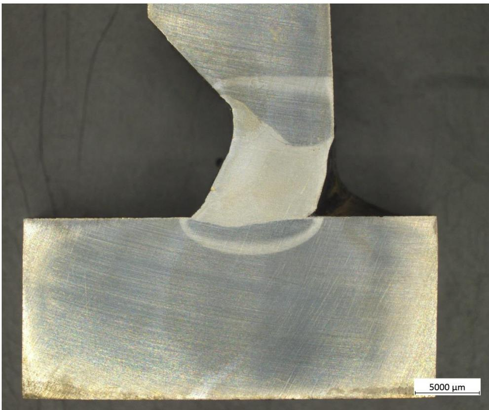
*Figure 29. Specimen welded at Huddig, half V-joint with land and 2,5mm gap.*
