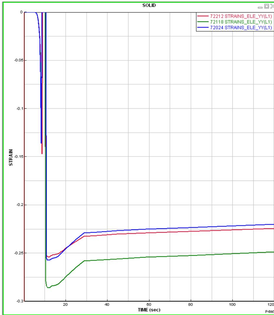
Figure 23. Continuous strain for elements in area most prone to form hot cracks for specimen welded with low aim.
