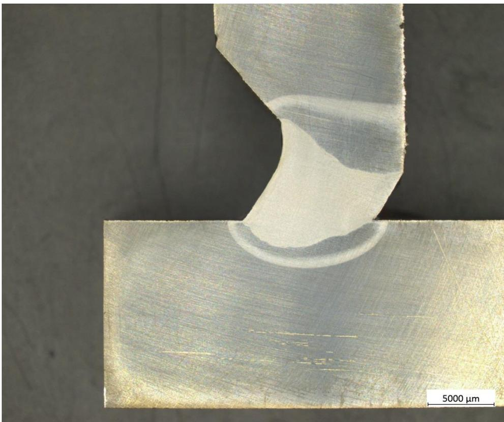
*Figure 27. Specimen welded at Huddig, half V-joint and 2,5mm gap.*
