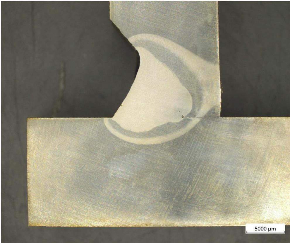
*Figure 28. Specimen welded at Huddig, half V-joint with land and 0mm gap.*
