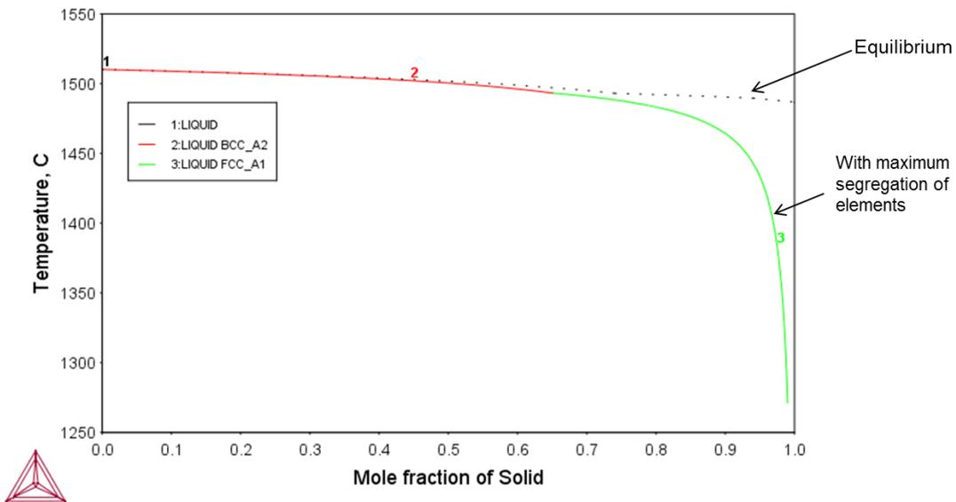
Figure 9 Solidification range of the same alloy used for calculations in Figure 8
