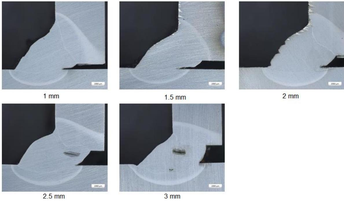
*Figure 5. Cross-sections from series welded with low aim.*
