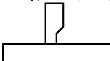
Figure 25. Illustration of joint preparation for half V-joint with land.
