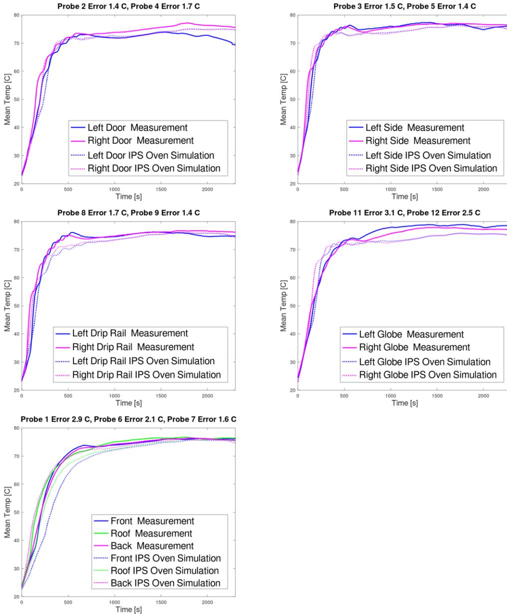
Figure 18 – Comparison of simulation results and measurements on the AB Volvo truck cab
