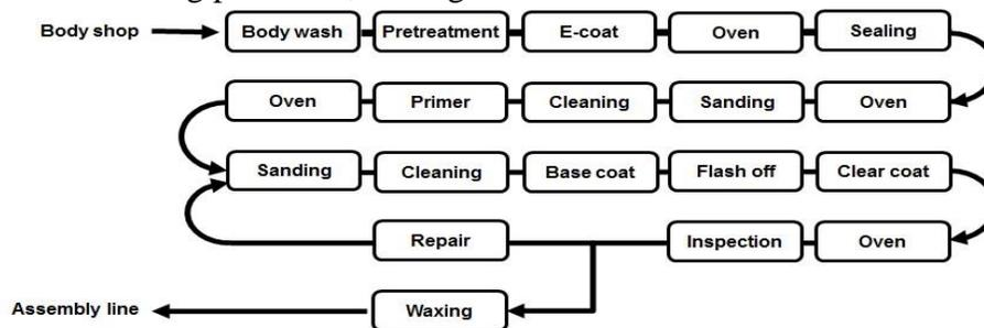
Figure 1. Process steps in a modern automotive paint shop.
