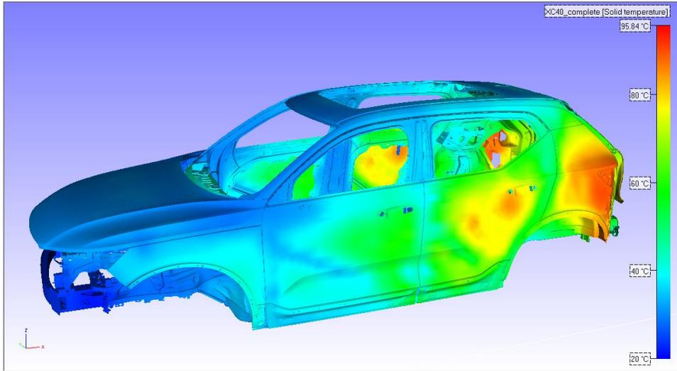
Figure 5 - Simulation result inside IPS Oven Simulation
