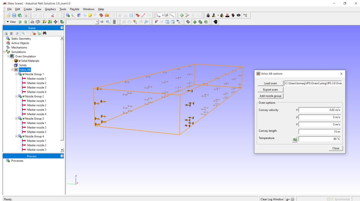
Figure 2 - Oven Setup with nozzles and properties
