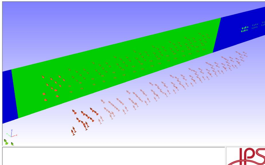
Figure 20 - One heating zone in the oven with the nozzles displayed.
