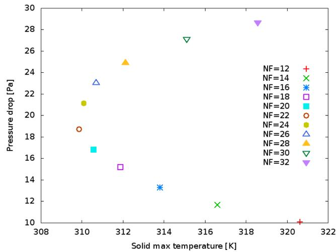
Figure 24 - Heat Sink Fin number optimization
