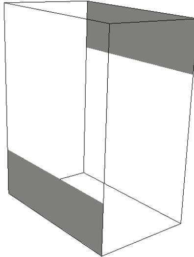
Figure 26 - Setup of the oven with inlet on top and outlet at the bottom
