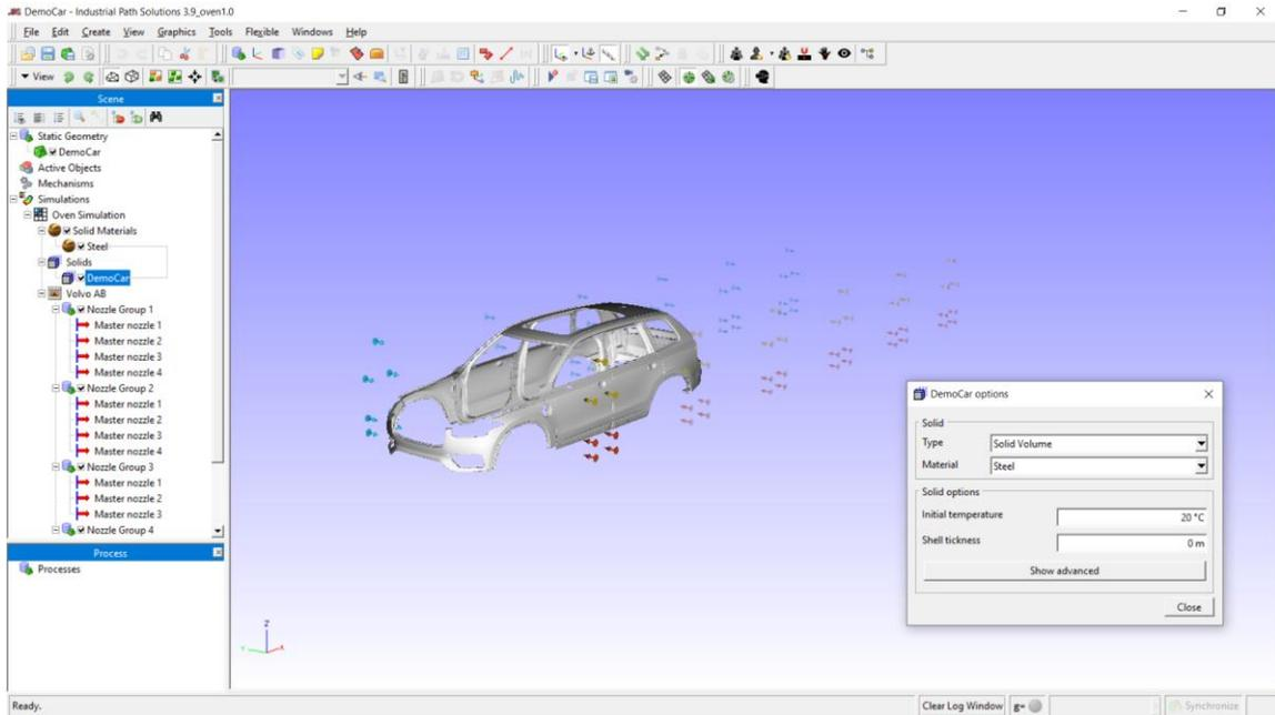
Figure 3 - Setup of object and material
