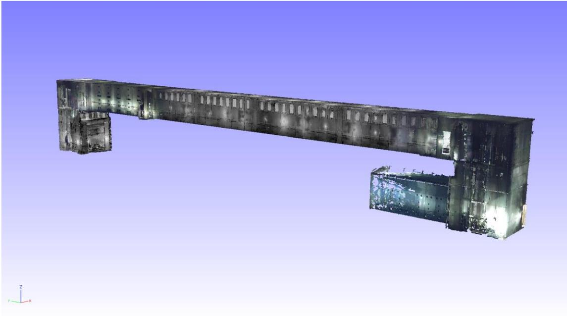
Figure 16 - Overview of the AB Volvo Umeå top coat oven, from 3D scan.
