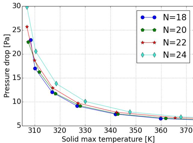
Figure 25 - Pareto front approximation for the heat sink design problem
