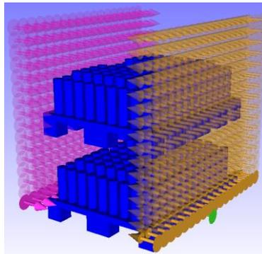
Figure 4 - Stationary objects inside a small oven with many nozzles
