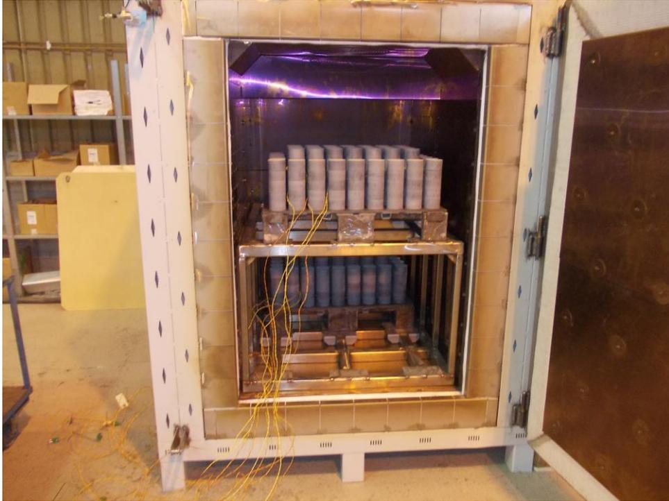
Figure 13 - ElectroHeat oven with zinc pucks used for validation
