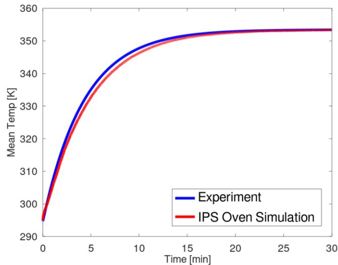
Figure 12 - Validation of the larger thermoplastic object
