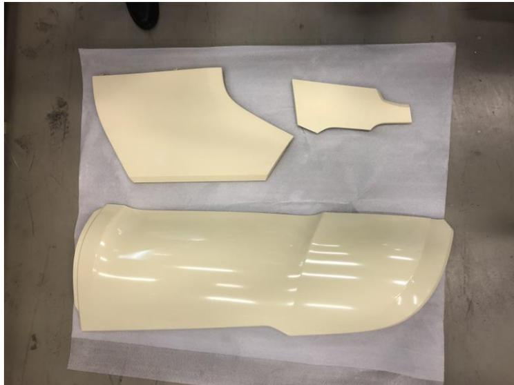
Figure 7 - Scania parts used for validation. The bottom part is steel, the other two pc/pet.
