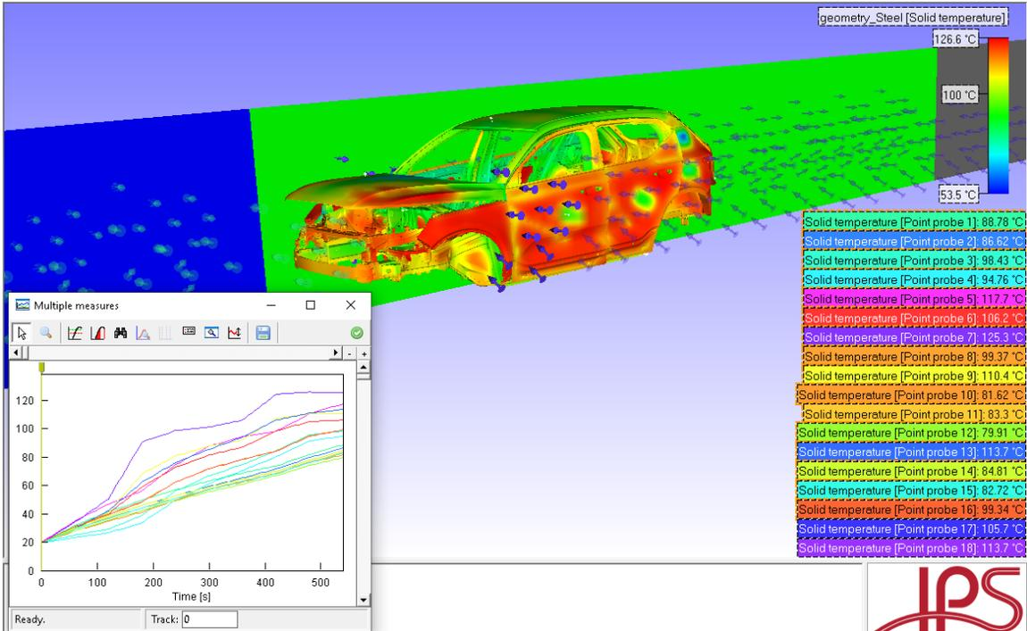
Figure 21 - Simulating an XC40 inside the Gent oven, with nozzles and probes.
