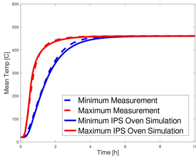
Figure 15 - Validation of the ElectroHeat oven
