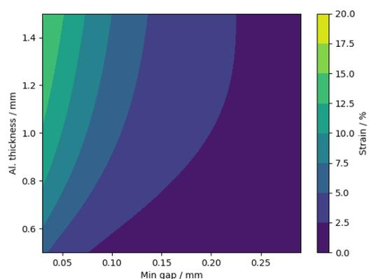
*Figure 22 - Guidelines in the form of a map of maximum strain of the adhesive after cooling.*
