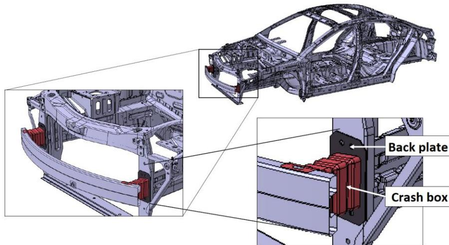
Figure 5 – Illustration of crash box and back plate in steel
