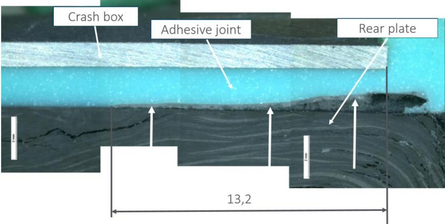
Figure 27 – Voids and crack like imperfections in the CFRP
