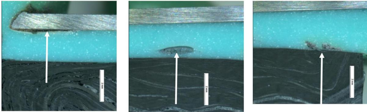
Figure 28 – Imperfections in a tensile tested crash box
