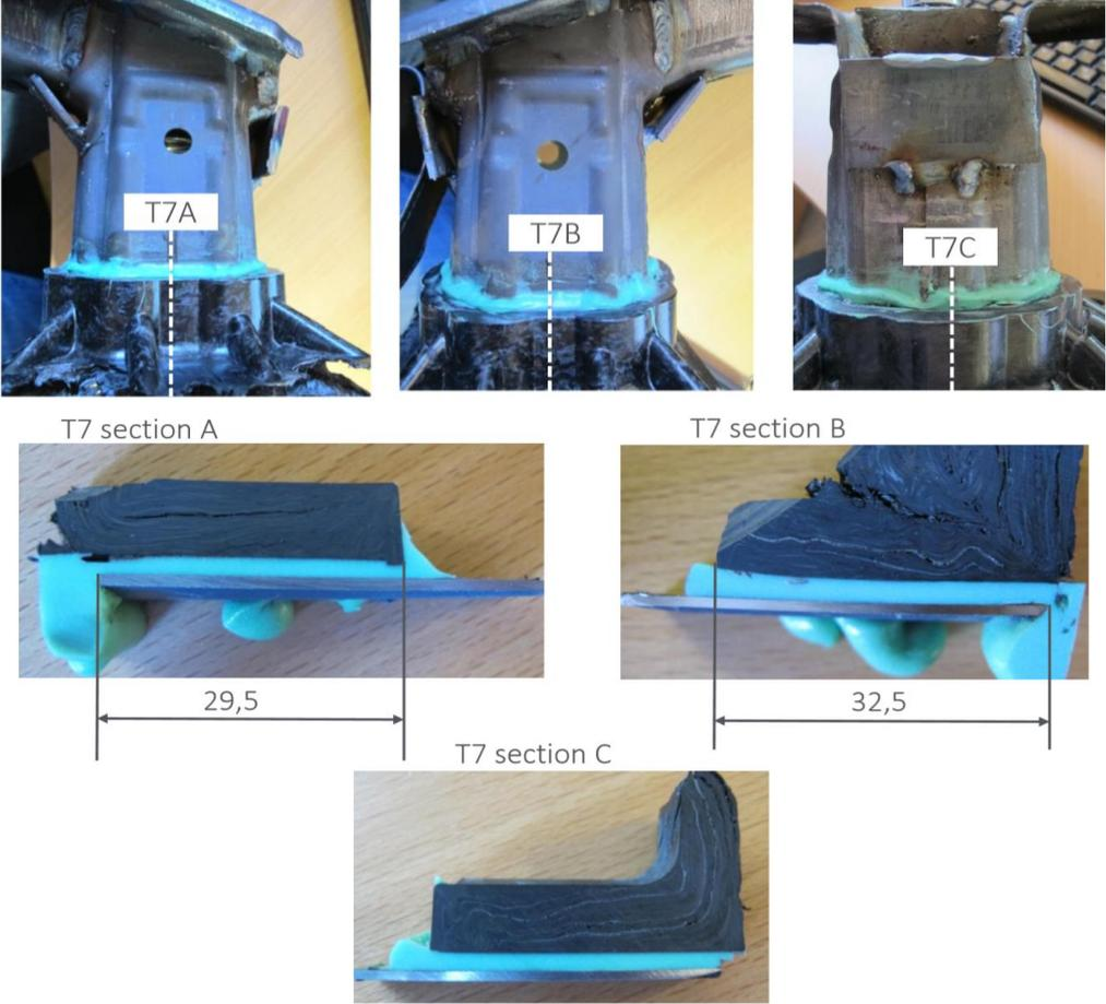
Figure 26 – Three cross sections of a tensile tested crash box
