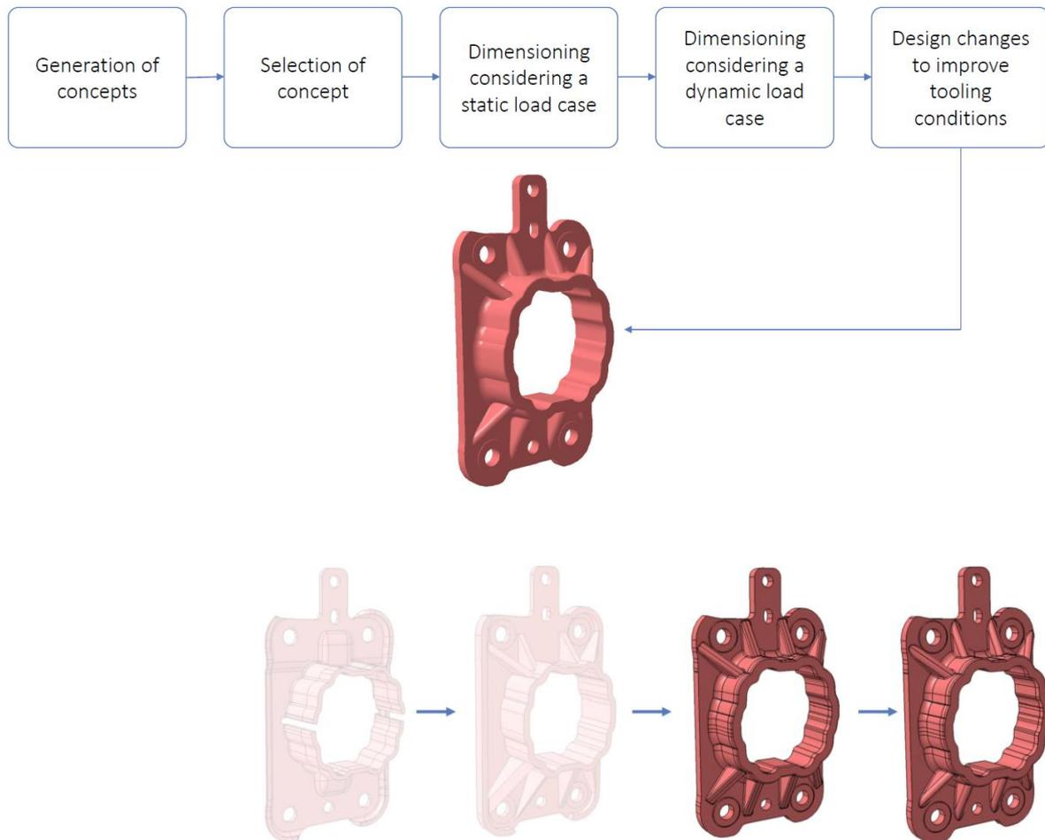
*Figure 7 - Design Procedure Overview – note that the back plate geometry changes for each iteration step.*
