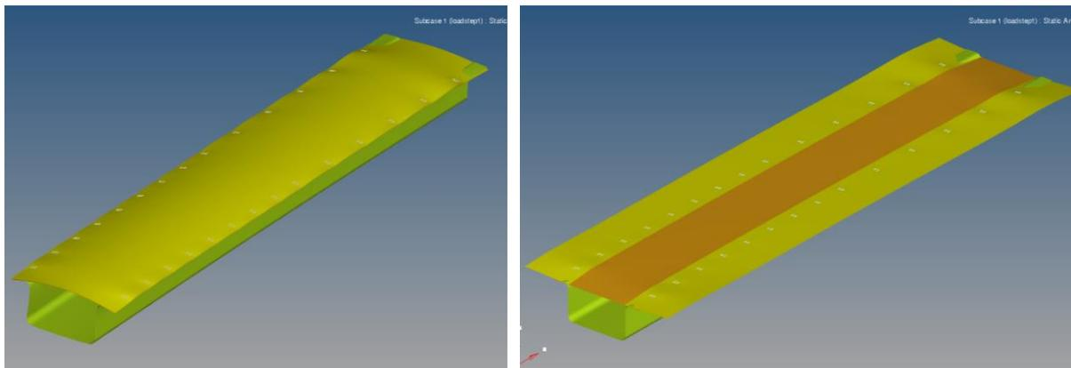
Figure 16 – Examples of simplified geometry used to evaluate deformations due to differences in thermal expansion coefficient.
