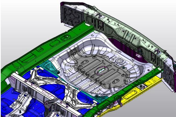
Figure 1 – Rear floor of Volvo V90
