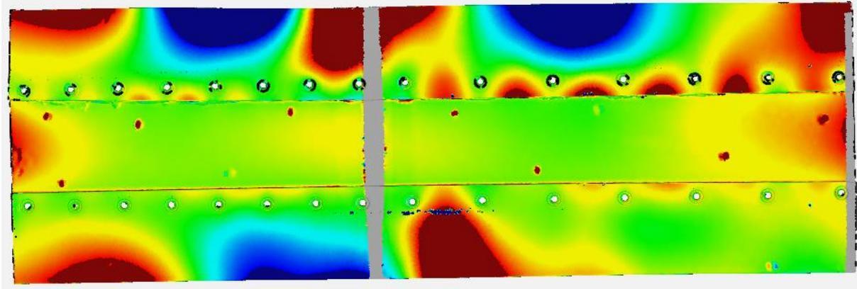
*Figure 17 – Comparison of geometries before and after adhesive curing (both at room temperature). Color map of distortions relative to the original shape prior to adhesive curing, green = same shape as before. The lower joint was without adhesive and show less distortion.*
