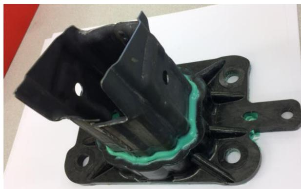
Figure 6 – The crash box and back plate produced with the final design
