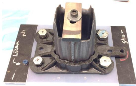
Figure 12 – Fixture used to fix the gap where the adhesive was later applied.
