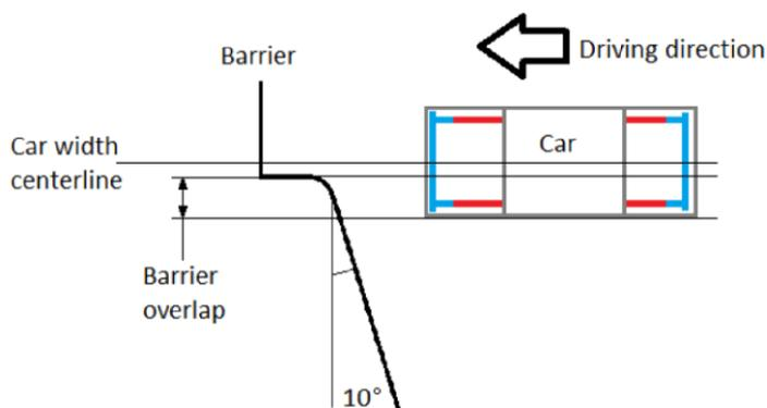
Figure 9 – RCAR Structural Test Setup [1,2]
