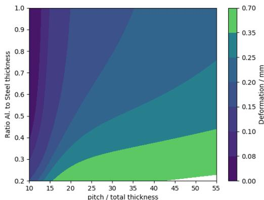
*Figure 21 - Guidelines in the form of a map of deformations of the joint at curing.*
