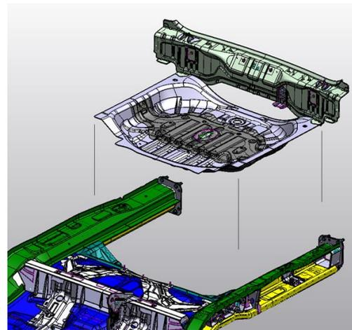
Figure 2 – Spare wheel housing detached from the rear floor
