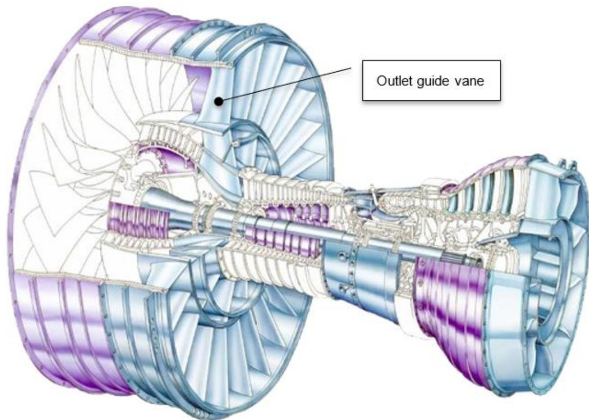
Figure 3 - *Outlet guide vanes in an aeroengine*
