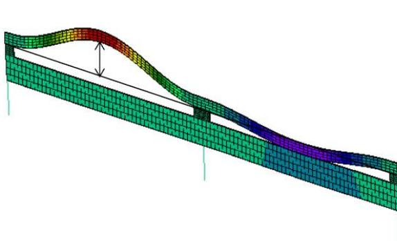
Figure 18 – Example of 2D simulation of maximum distortion for heating cycles from 20 → 180C.
