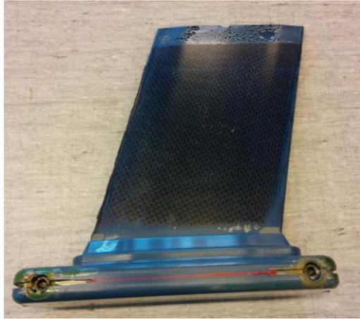
Figure 24 - Titanium bracket and composite vane manufactured and bonded by co-curing.
