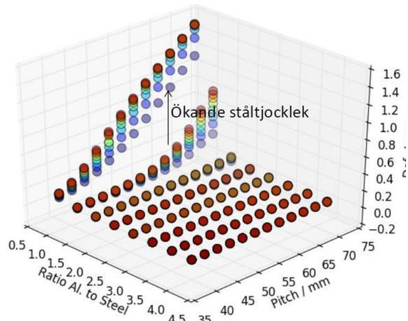
Figure 19 – Resulting maximum distortion as a function of sheet thickness ratio and pitch distance
