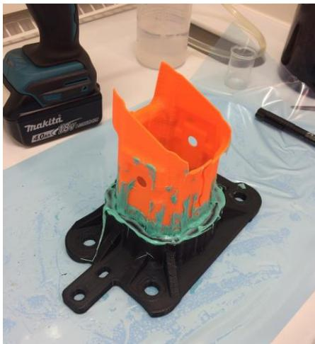
Figure 11 – 3D printed back plate and crash box.
