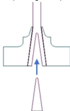
*Figure 23 - Cone shaped pocket with a wedge in the composite vane will act as a mechanical locking*
