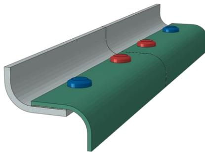
*Figure 20 - 3D model of Al-Fe joint including an adhesive.*
