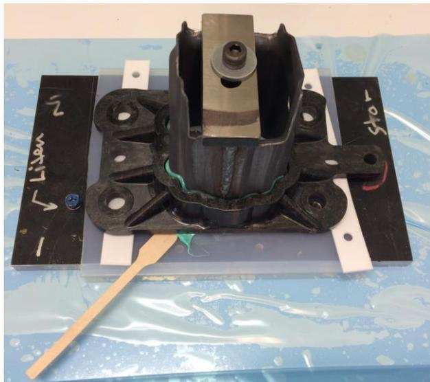
Figure 13 – Procedure used to apply adhesive.
