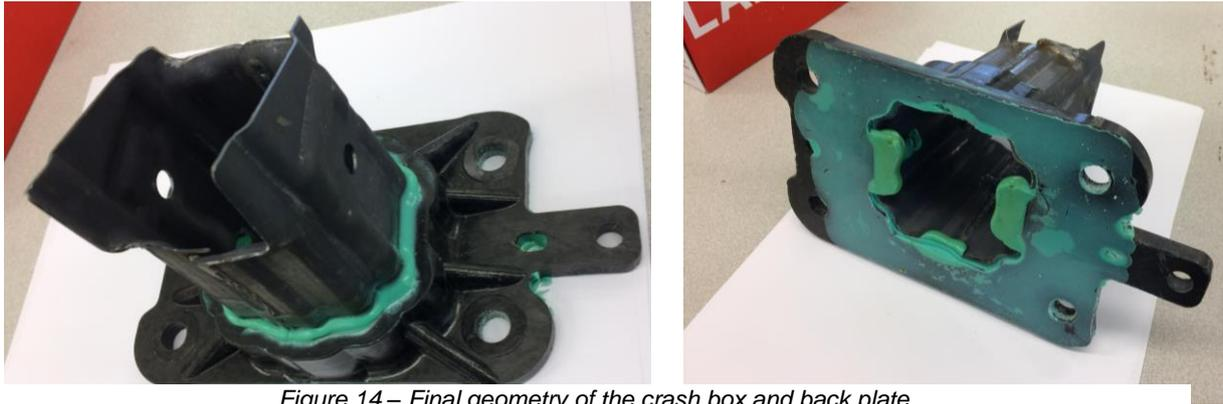
Figure 14 – Final geometry of the crash box and back plate.
