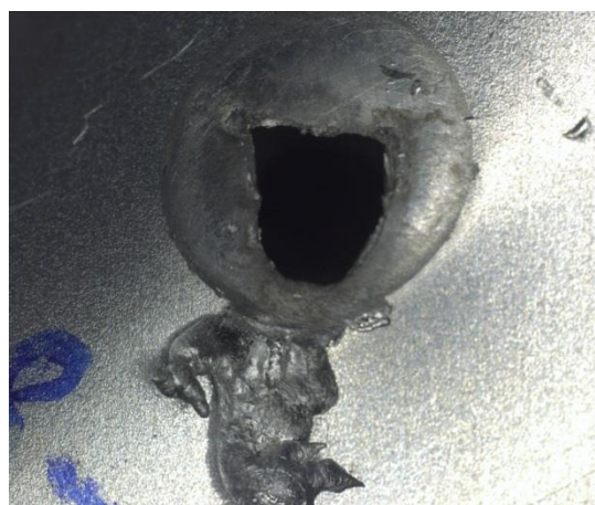
Figure 14. Surface spatter from welding with TiB_2 -coated caps and a current level of 10 kA.
