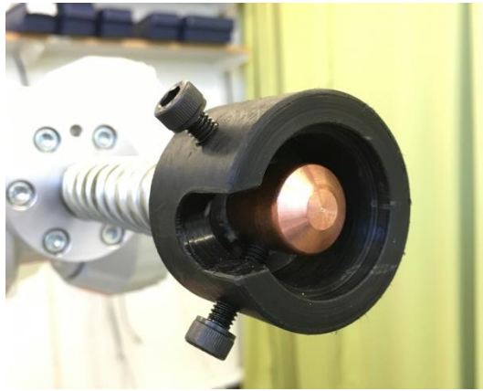
Figure 8. A specialized holder for the caps was developed in order to easily move the target
