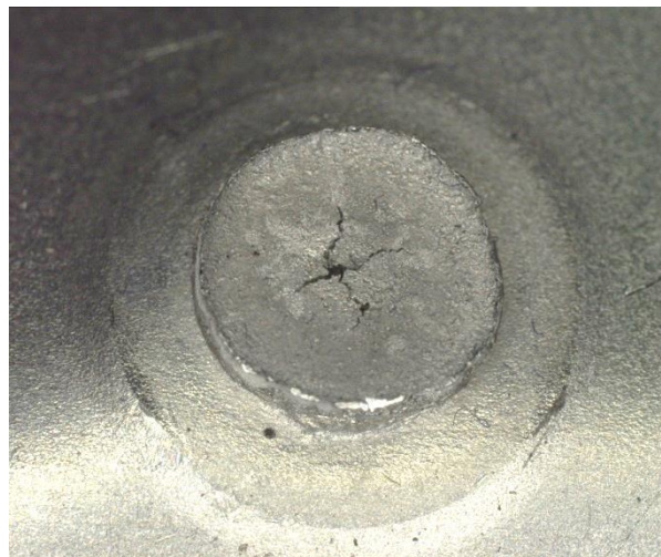
Figure 25. Nugget welded with Rh-coated solid Mo-caps and process parameters as presented in Table 4 .
