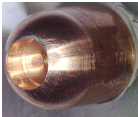
Figure 19. Cu-cap after the tungsten plug got stuck to the sheet.
