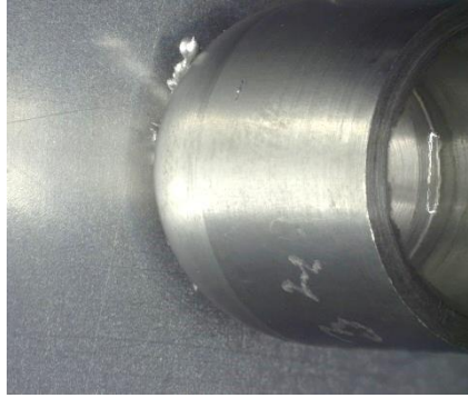
Figure 16. Solid Mo-cap stuck to upper sheet.
