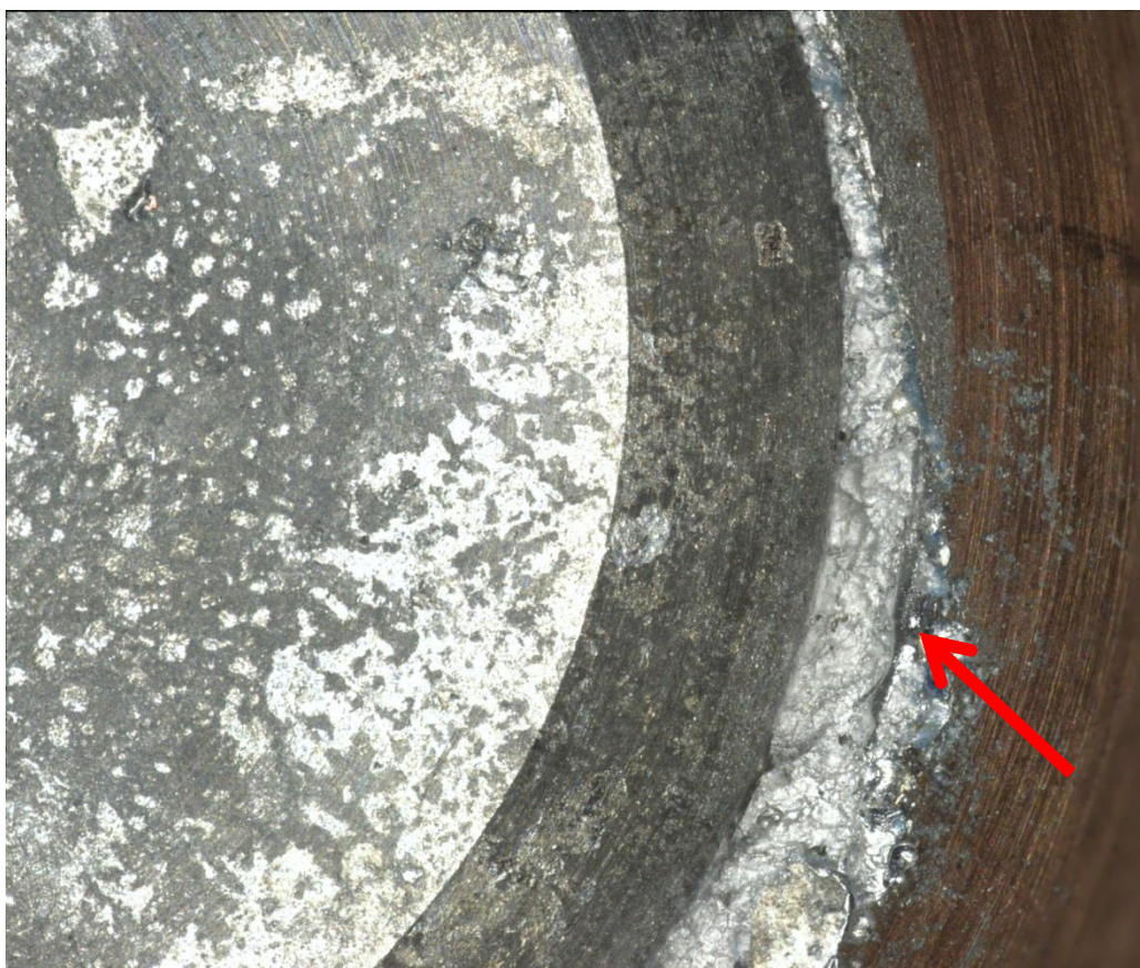
Figure 20. Crack between W-plug and Cu-cap after 54 spots. Heavily wear of the contact area can also be seen.
