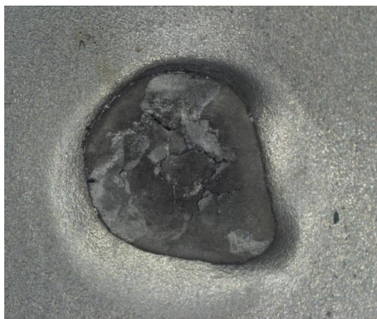
Figure 21. Undersized nugget with cracks in the centre. Welded with 15,3 kA.
