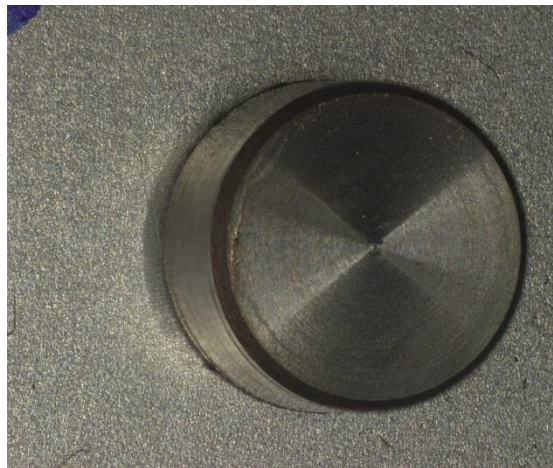
Figure 24. Mo-plug from Rh-coated Cu-cap stuck in the sheet.
