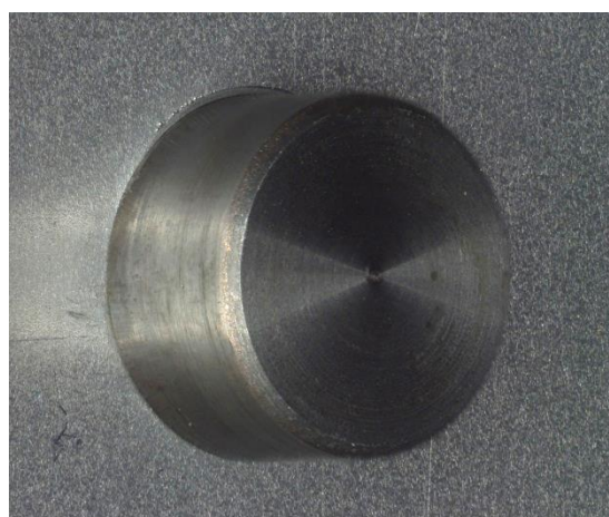
Figure 23. Mo-plug stuck to lower sheet. Welded with a current of 15,9 kA.
