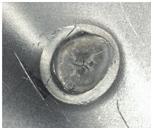
Figure 13. Nugget from welding with TiB_2 -coated caps and a current level of 9 kA, other parameters kept as presented in Table 3. Cracks can be seen in the centre of the nugget.
