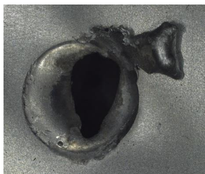
Figure 15. Surface spatter from spot welded with solid un-coated Mo-cap with weld current at 12 kA.
