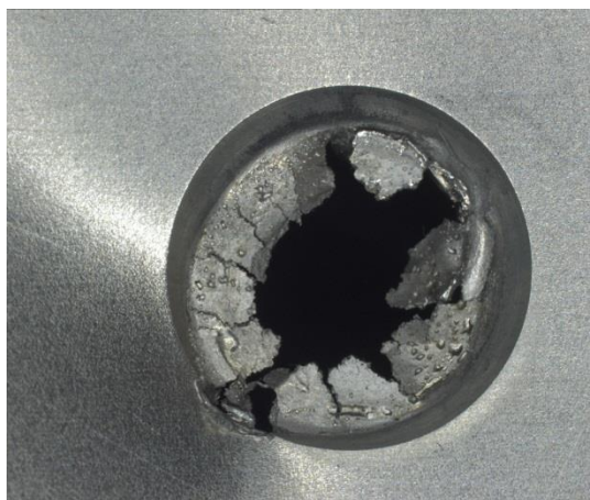
Figure 11. Hole through sheets from welding with TiB_2 -coated Mo-caps and process parameters as presented in Table 3.
