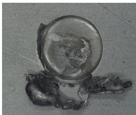
Figure 22. Surface spatter from sot welded with Cu-caps with Mo-plug. Current at 15,6 kA.
