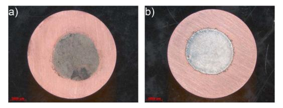
*Figure 4: The effect of exchanging the electrolyte on deposit quality: a) no exchange of electrolyte, and b) with exchange of electrolyte.*
