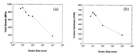
Figure 1: Grain size dependence of Vickers hardness and yield strength of nickel at room temperature [El-Sherik and Erb in "Nickel-Cobalt 97 – Vol. IV, Applications and Materials Performance", The Metallurgical Society of CIM, Montreal, (1997) 257].
