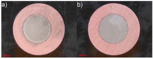
Figure 5: Deposits achieved by pulsed electrodeposition in a confined bath setup: a) pulse on-time of 10 ms, and b) pulse on-time of 1 s.
