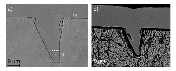
Fig. 6: Cross-section optical micrographs of a scratch repaired with LECD of nickel: a) without etching (a black line is added to visualize the interface; the locations of the EBSD orientation maps (Fig 7) are marked but are not in the right size), and b) overview with heavily etched Cu-substrate.
