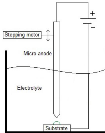
Figure 2: Scheme of the LECD experimental setup as used for deposition of microfeatures.
