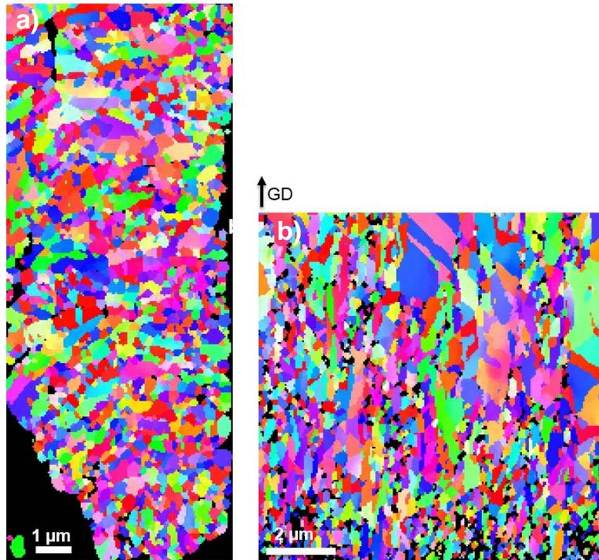
Fig. 7: EBSD orientation maps of the deposit as marked in Fig. 6a: a) in the tip of the scratch (maximum noise control applied), and b) in the neighborhood of the scratch.
