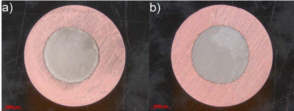
Figure 5: Deposits achieved by pulsed electrodeposition in a confined bath setup: a) pulse on-time of 10 ms, and b) pulse on-time of 1 s.
