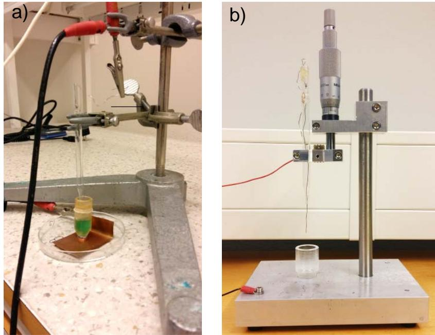
Figure 3: Experimental setup used in the confined bath concept: a) container placed directly onto the substrate (use of rubber sealing ring), b) container screwed onto the stage (use of rubber sealing ring, a partly encapsulated microanode is mounted).
