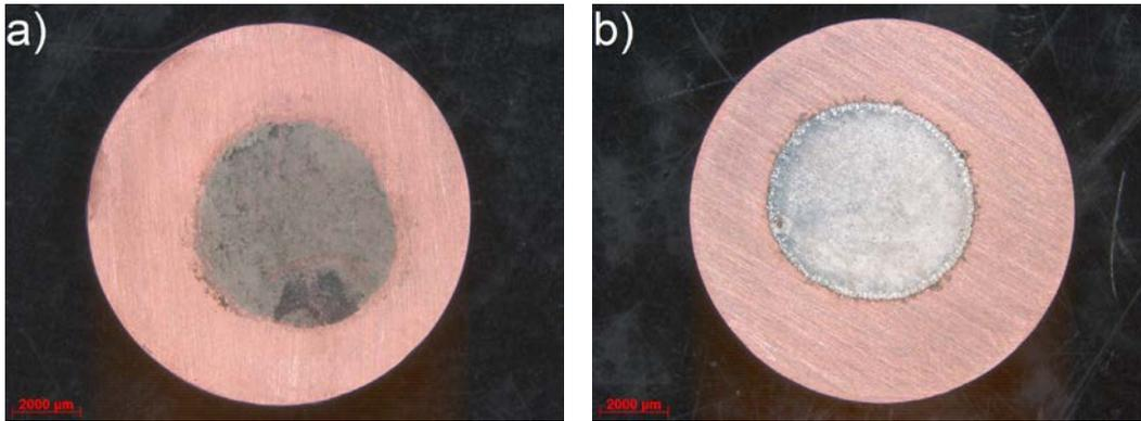
Figure 4: The effect of exchanging the electrolyte on deposit quality: a) no exchange of electrolyte, and b) with exchange of electrolyte.
