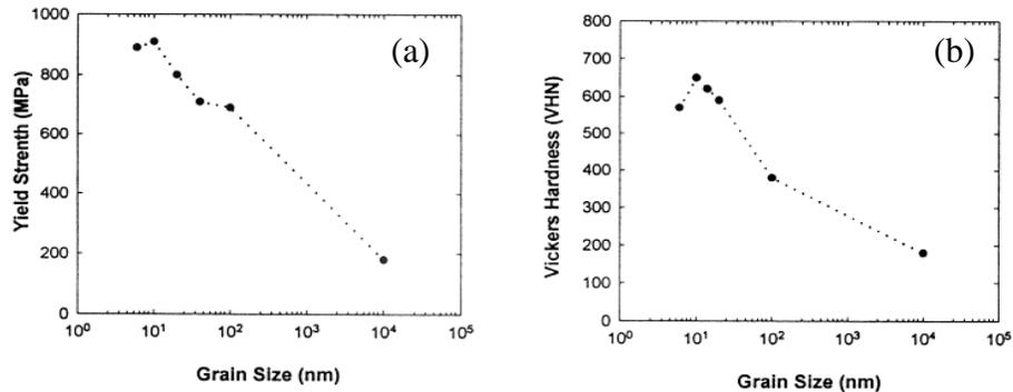
*Figure 1: Grain size dependence of Vickers hardness and yield strength of nickel at room temperature [El-Sherik and Erb in “*Nickel-Cobalt 97 – Vol. IV, Applications and Materials Performance*”, The Metallurgical Society of CIM, Montreal, (1997) 257].*
