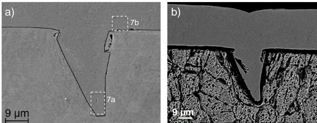
Fig. 6: Cross-section optical micrographs of a scratch repaired with LECD of nickel: a) without etching (a black line is added to visualize the interface; the locations of the EBSD orientation maps (Fig 7) are marked but are not in the right size), and b) overview with heavily etched Cu-substrate.
