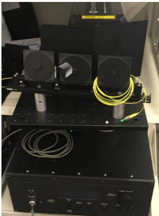
Figure 5. The laser of the FP-system, the laser light is guided to the work piece, via multimode fibers.
