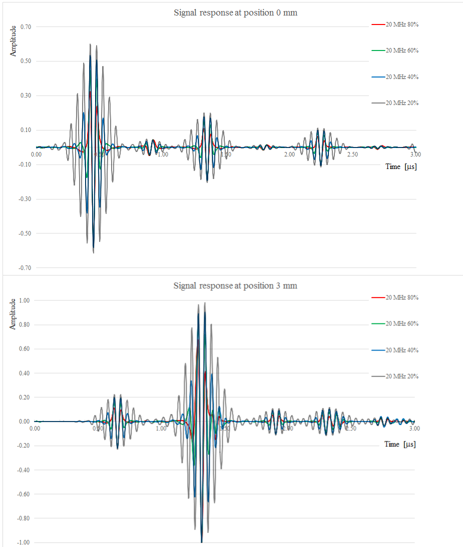
Figure 23. The signal response as function of applied bandwidth, when the detection is on opposite side directly beneath the LUS source (the upper figure) and position x=3 mm (the lower figure).
