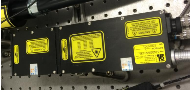
Figure 4. Quantel Ultra 100 BigSky IR generation laser, commonly referred to as the small generation laser.
