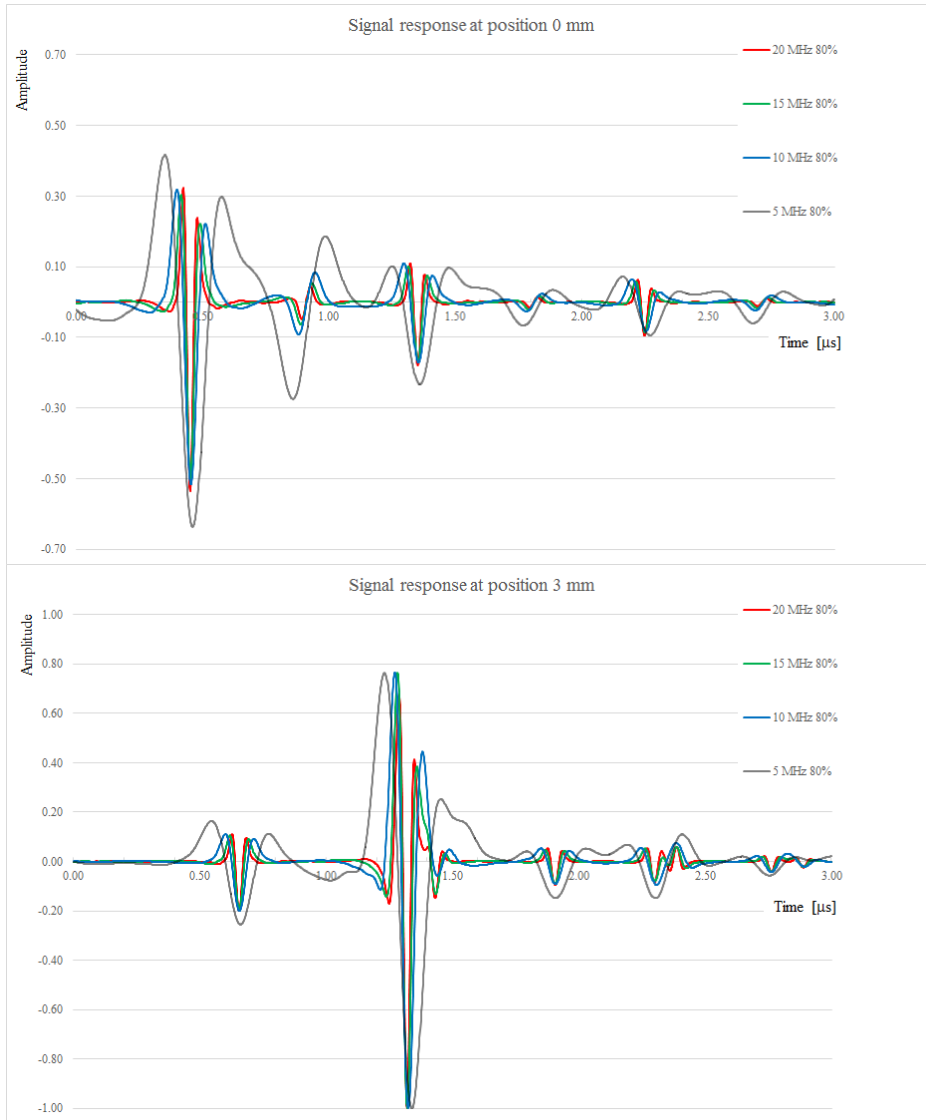
Figure 22. The signal response as function of centre frequency, when the detection is on opposite side directly beneath the LUS source (the upper figure) and position x=3 mm (the lower figure).
