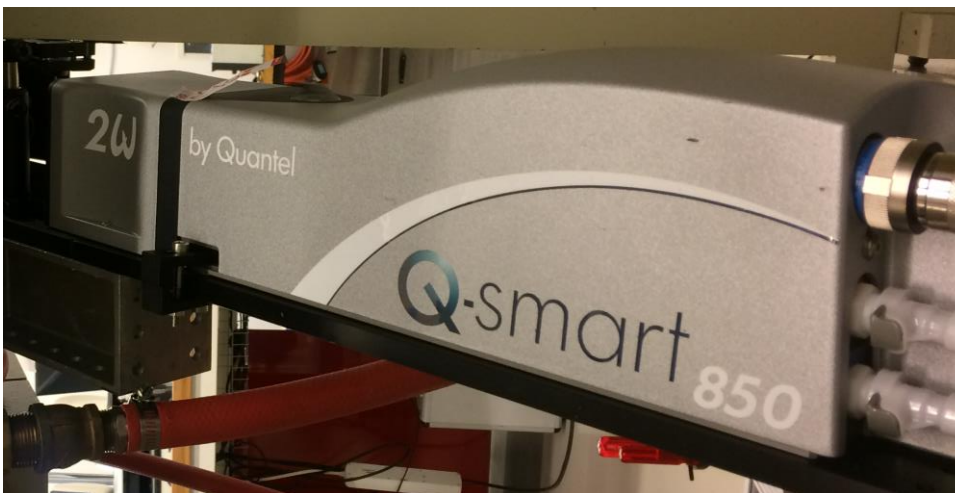
Figure 7. The green generation laser from Quantel.
