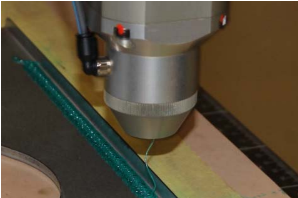
Bild 6 New application technique, e-swirl has been evaluated
