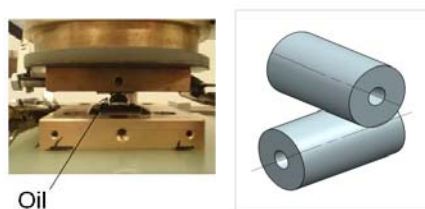
Figure 2. Experimental set up for the Fretting test.
