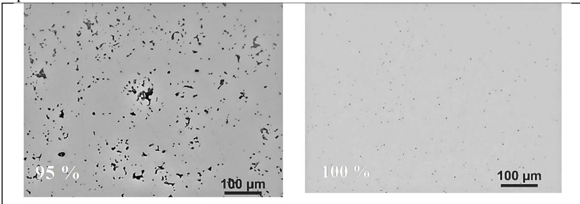
Fig 6 Example of pore distribution before (a) and after HIP operation(b).
