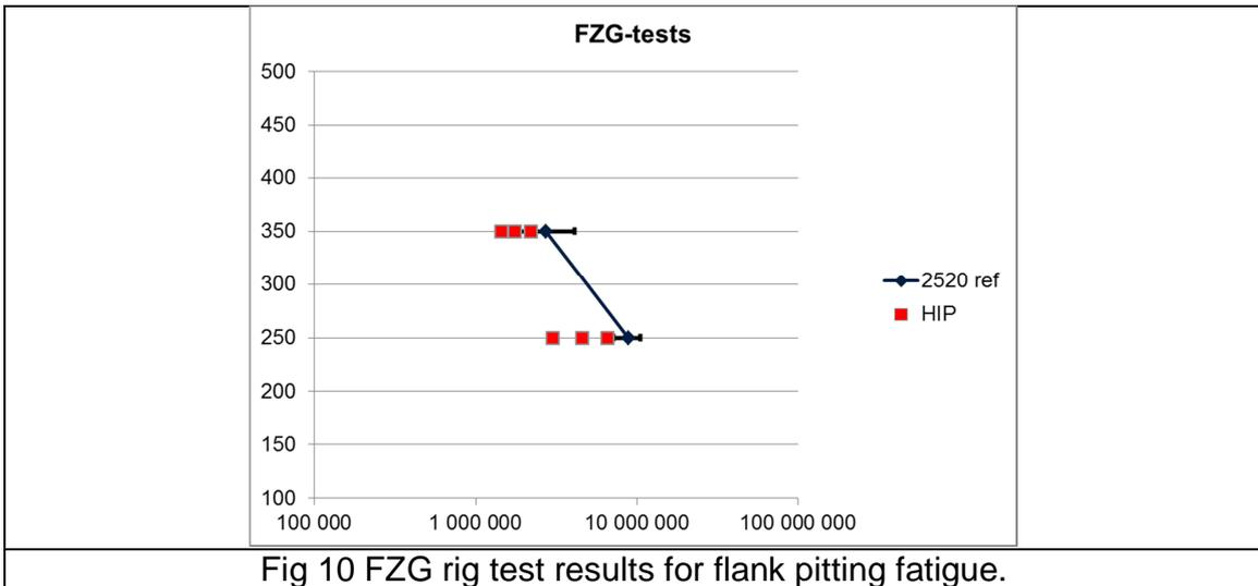
Fig 10 FZG rig test results for flank pitting fatigue.
