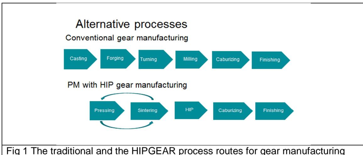
Fig 1 The traditional and the HIPGEAR process routes for gear manufacturing
