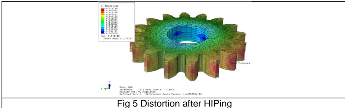
**Fig 5 Distortion after HIPing**
