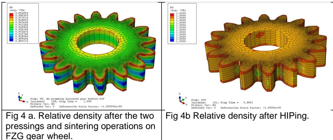
Fig 4 a. Relative density after the two pressings and sintering operations on FZG gear wheel.
