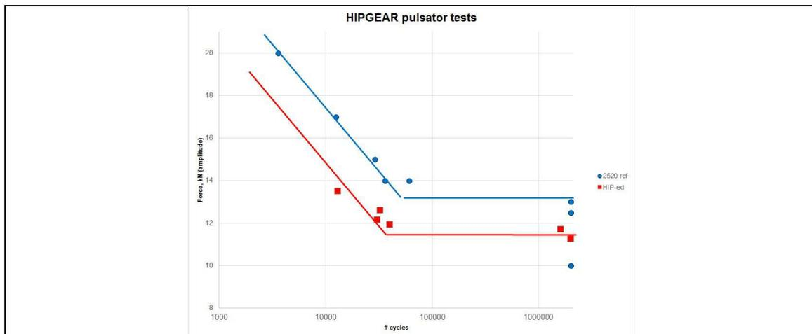
Fig 11 Tooth root bending fatigue tests.
