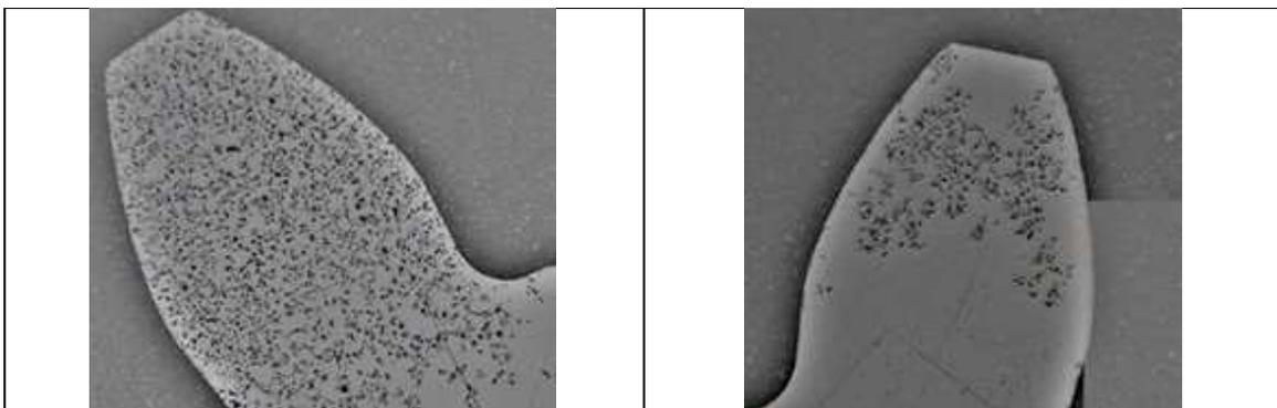
Fig 7a Example of pores after HIP with open porosity
