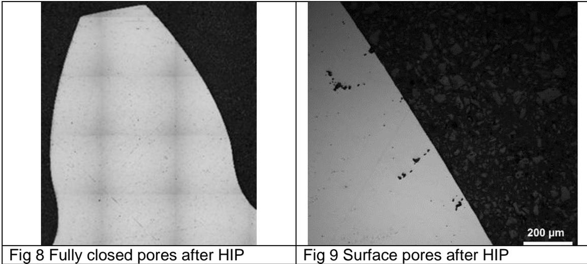
Fig 8 Fully closed pores after HIP
