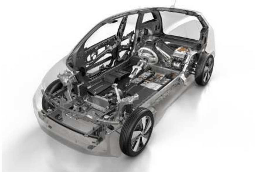
Fig. 1 Cross-section of the BMW i3 with a complete composite cabin
