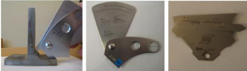
Figure 9: a) Measurement principle revision gauge, a-height [mm], b) revision gauge – calculates a-height from measured position of weld toe, c) production gauge, measure a-height directly on weld ridge (45 deg from base plate).
