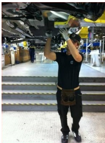
Figure 1: Manual assembly of aero panels under a vehicle as it is performed today
