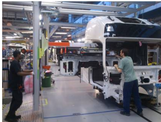
Figure 7: The assembly of huge interior in a truck cab as it is performed today
