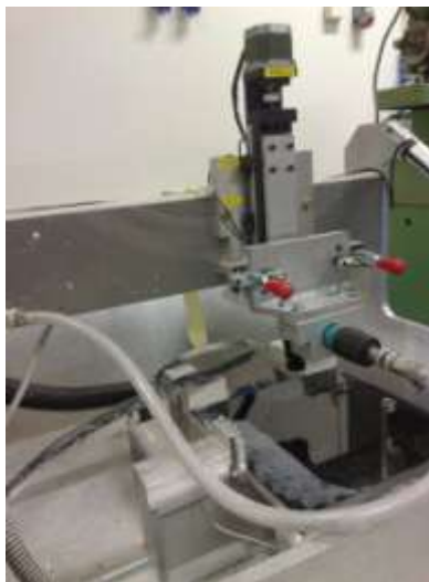
The polishing-rig developed at Volvo Cars where different clear coats and polishing strategies can be tested in a systematic way.
