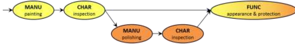
Figure 1: Flow chart to illustrate the steps towards ‘defect free’ coatings; MANU – manufacturing, CHAR – characterization, and FUNC – function.
