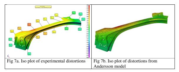
A shell element FE-model was generated from the CAD models of the components of the A-pillar and simulations were performed with the Andersson model for laser beam welding. It was considered unrealistic for the presently available computer power to use the fully coupled model. The simulation was completed by simplified modeling of the spot welds which joined by sheets. The spot welds were modeled as a cylinder around the center of the spot weld.
