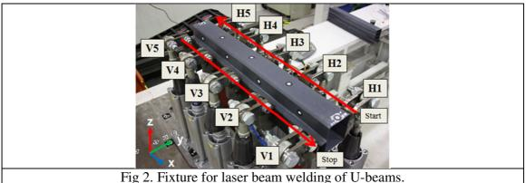
A Nd-YAG laser with peak power of 4kW was used for the trials. All trials were made at peak power but different welding speeds to alter heat input per unit length, welding patterns and continuous and stitch welding was applied. Different modes of releasing the fixturing points was also investigated.
