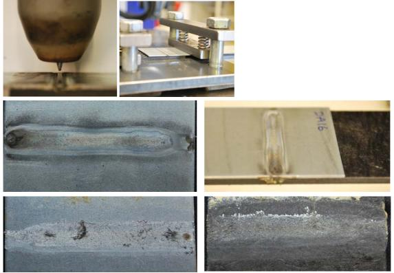
Joining of thermoplastic composite with short fibres to zinc coated steel Heat source TIG with constricted arc: EWM forceTIG, Steel with sheet thickness 1.2mm and with approx.  $7\mu m$  zinc coating Travel speed: 0.85m/min Shear-tensile test:  $F_m$ : 4.0kN Joint fracture area:  $\approx 288 mm^2$  (48 x 6) Shear strength 13.9MPa
