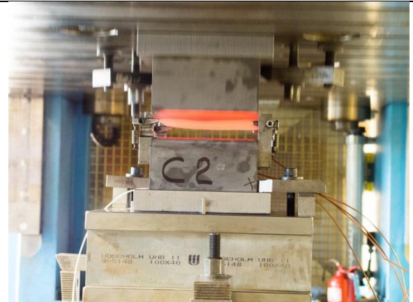
(b) Hot boron steel blank during pressing trials with an experimental tool at AP&T Blidsberg
