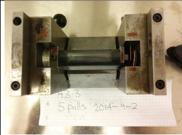
(c) Pin showing used contact surface after five drawing tests
