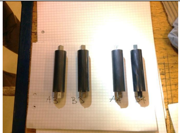
(b) PVD coated drawing pins manufactured by AP&T and Oerlikon using tool material supplied by Uddeholm.
