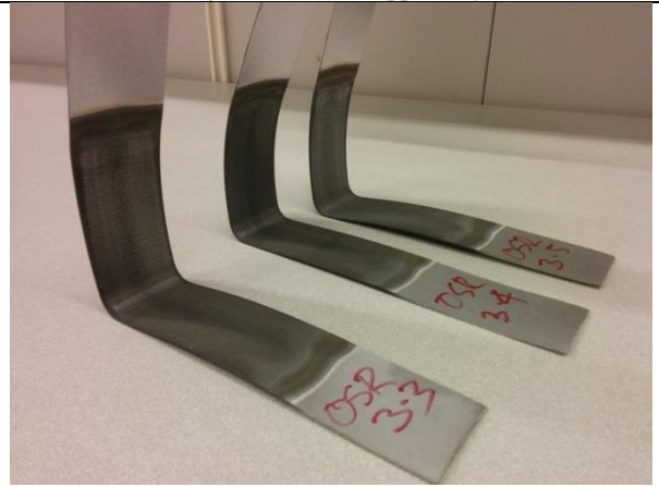
(d) Final bent and drawn Al-Si coated Boron steel samples
