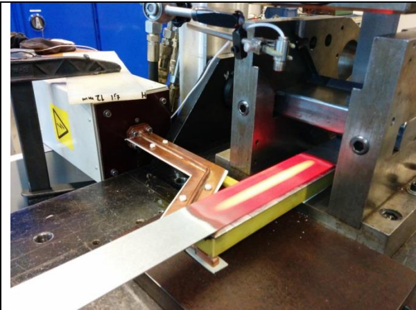
(a) Al-Si coated Boron steel during in-situ heating in the bending-under-tension machine at Swerea KIMAB
