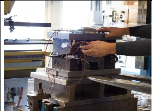
(a) Instrumented press tool developed in the project for measuring the temperature of tool and blank during pilot plant hot pressing trials
