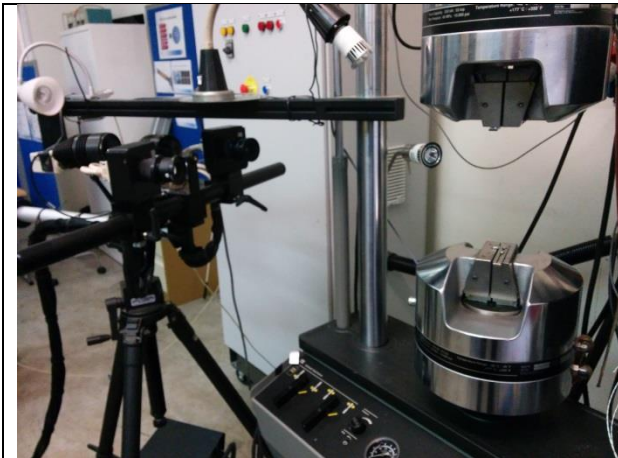
(a) Hot tensile testing system using the Aramis strain measurement system for evaluating deformation behavior at pressing temperature, developed at IUC Olofström
