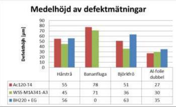
Figure 4. Measured defects caused by various particles.
