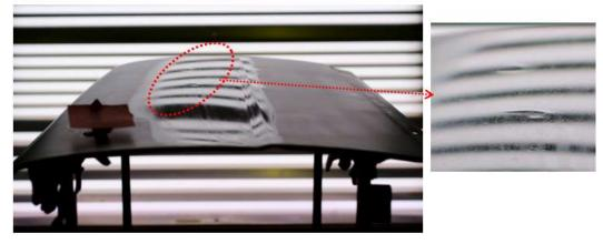
Figure 1. The figure shows a rejected outer panel (car door) which has been formed with two strands of hairs placed on the stamp. The defects are visualised by the light. The detail has a blanking liquid applied, which simulates varnishing. The stripes are a reflection phenomenon which is caused by the illumination.
