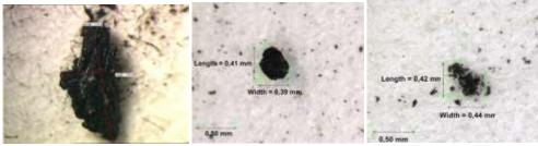
Figure 5. Examples of particles collected on a filter from the press line.
