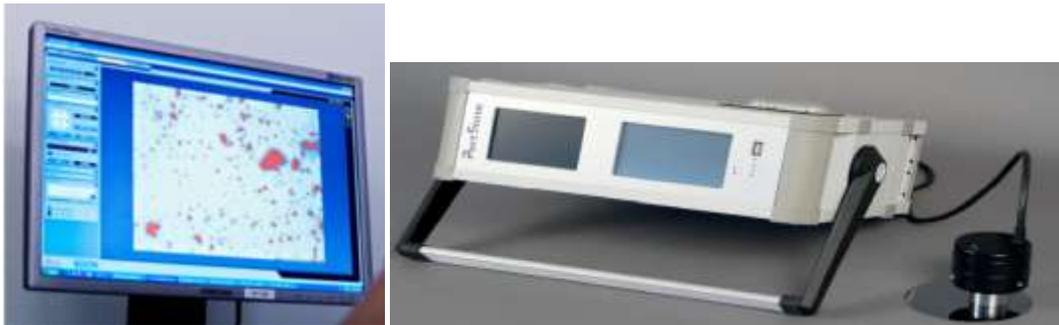
Figure 2. Particle analysis with image processing and particle counter PartSens.
