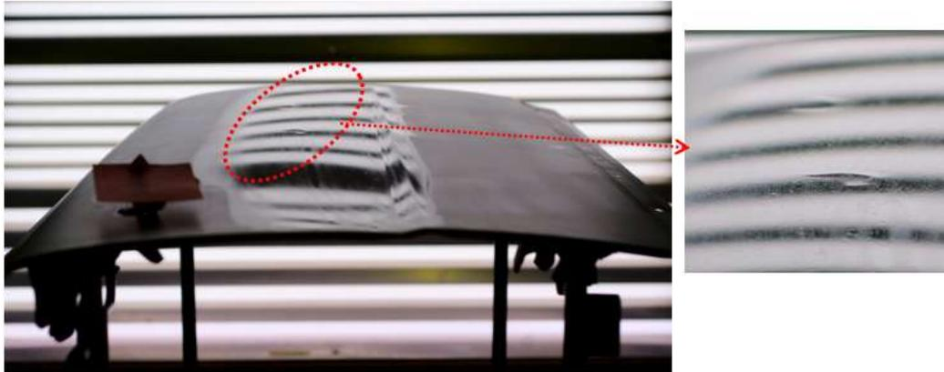
Figure 1. The figure shows a rejected outer panel (car door) which has been formed with two strands of hairs placed on the stamp. The defects are visualised by the light. The detail has a blanking liquid applied, which simulates varnishing. The stripes are a reflection phenomenon which is caused by the illumination.
