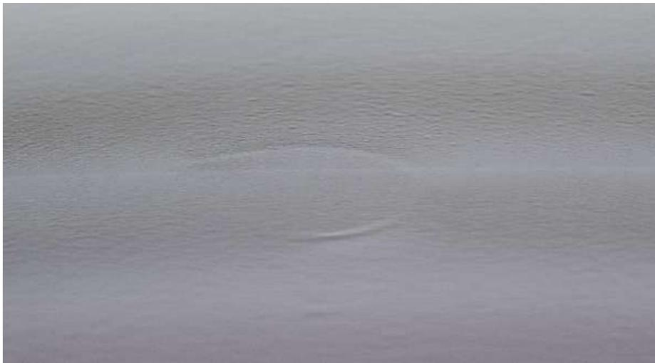
Defect on a stamped outer panel of a car door caused by a strand of hair
