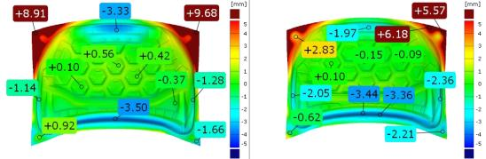
Figure 12 Spring back with Barlat `89 (left) and BBC2005 (right).
