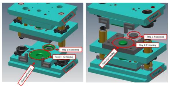
Figure 10 Layout of the semi industrial punching tool that was used in the project
