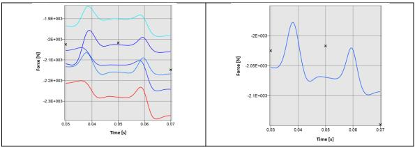
Figure 13 The picture on the left shows the different outcomes of the FE simulations with variable friction (iteration 1). The crosses represent the experimental values. The picture to the right shows the optimized solution of Shear-cap model.
