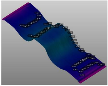
Figure 7 Simulated strains for the formed sheet metal component after one of the forming stations before trimming
