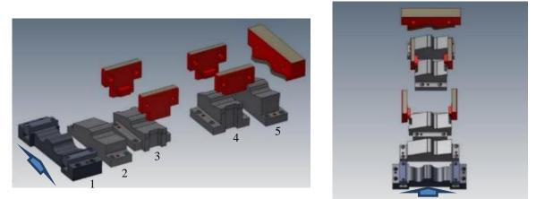
Figure 9 Layout of the semi industrial trimming tool that was used in the project
