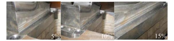
Figure 17 Example results regarding formation of burrs and slivers in trimming with different clearance (5, 10 or 15% of sheet thickness)
