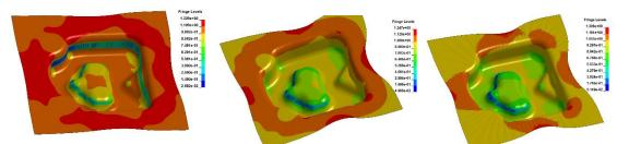
Figure 5 Thickness distribution in parts of the three evaluated aluminium alloys
