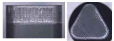
Figure 16 Example results regarding galling on trimming edges on punching tool
