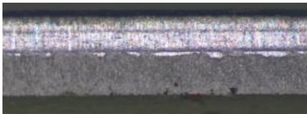
Figure 18 Example results regarding quality of punched part. Burrs that have been formed and still are attached to the part are also visible
