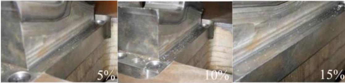
Figure 17 Example results regarding formation of burrs and slivers in trimming with different clearance (5, 10 or 15% of sheet thickness)
