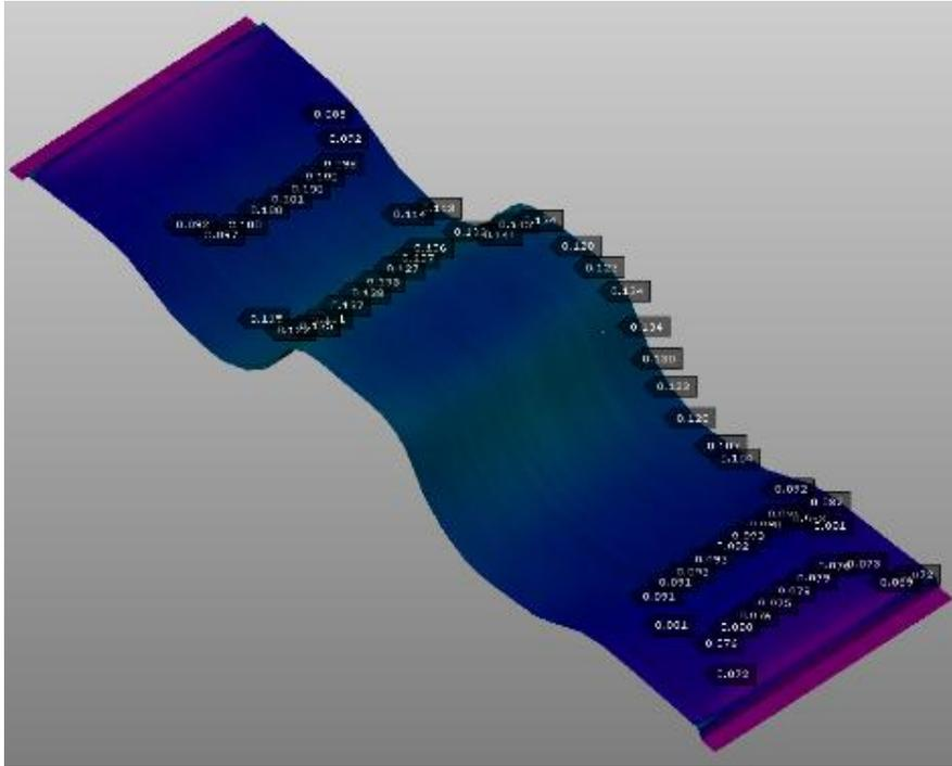
Figure 7 Simulated strains for the formed sheet metal component after one of the forming stations before trimming
