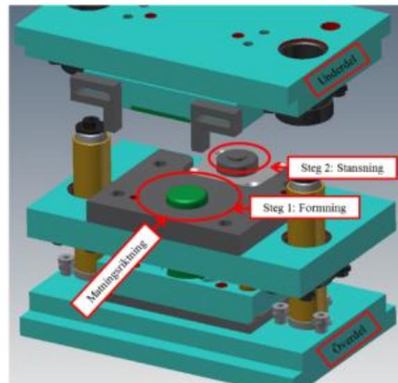
Figure 10 Layout of the semi industrial punching tool that was used in the project
