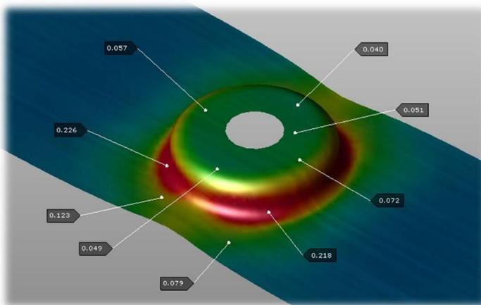
Figure 8 Simulated strains for the formed sheet metal component after the forming stations before punching
