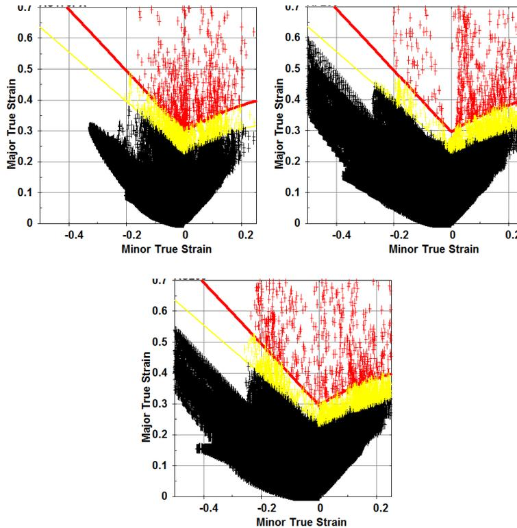
Figure 6 Forming limit diagrams for the three different aluminium alloys
