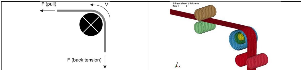
Figure 3 The picture to the left shows schematically the BUT experiment. The picture to the right shows the FE model that was used for calibration. It shows four freely rotating tools that reduces oscillation under tensile and three different radii that can gradually be exchanged for the calibration of the friction model.
