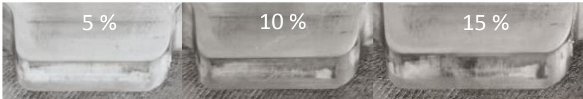
Figure 15 Example results regarding galling on trimming edges on trimming tool with different clearance (5, 10 or 15% of sheet thickness)
