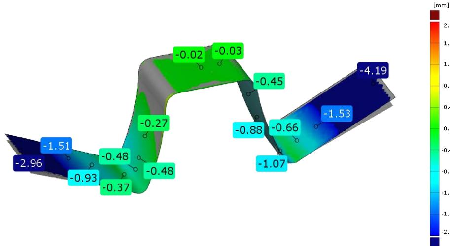
Figure 11 Deviation between the scanned geometry and results from simulation after spring back.
