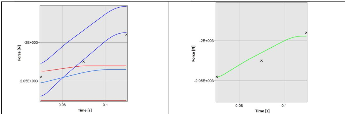
Figure 14 The picture on the left shows the different outcomes of the FE simulations with variable friction (iteration 1). The crosses represent the experimental values. The picture to the right shows the optimized solution of Emmen's model.
