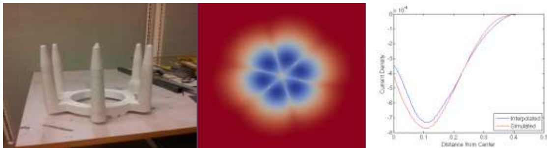
Figure 6. The ABB G1 applicator with six electrodes (left). The ion charge density between bell and target (middle). A comparison between the simulated and measured current density on a plate under the applicator (right).
