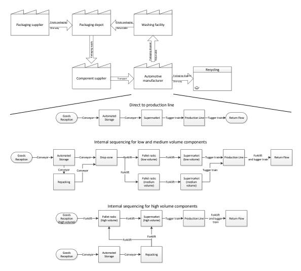
Figure 3. Overview of the supply chain and the materials flow types for the components in one of the plants covered in the analytical model
