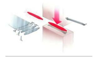
Figure 1. Illustration of the press hardening technique.
