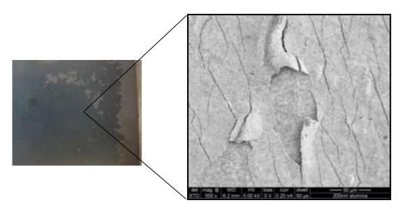
Figure 2. Macroscopical and microscopical image of loose oxide formed on the steel surface during hot stamping of uncoated steel.
