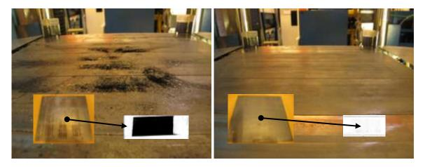
Figure 3. Hot stamping of non-pretreated reference material (left) as well as pre-treated material (right), the oxides showing very poor and excellent adhesion, respectively. The images show the tool surface after hot stamping and the amount of oxide that has flaked off from the blanks, as well as the produced blanks and the tape tests.
