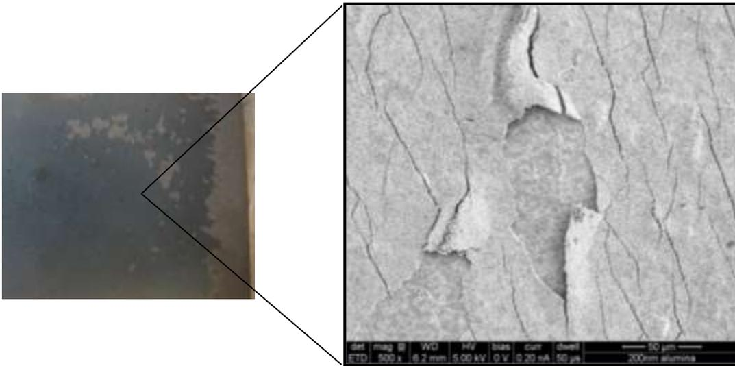
*Figure 2. Macroscopical and microscopical image of loose oxide formed on the steel surface during hot stamping of uncoated steel.*
