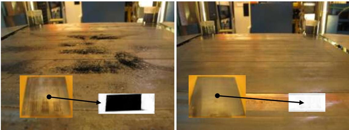
*Figure 3. Hot stamping of non-pretreated reference material (left) as well as pre-treated material (right), the oxides showing very poor and excellent adhesion, respectively. The images show the tool surface after hot stamping and the amount of oxide that has flaked off from the blanks, as well as the produced blanks and the tape tests.*
