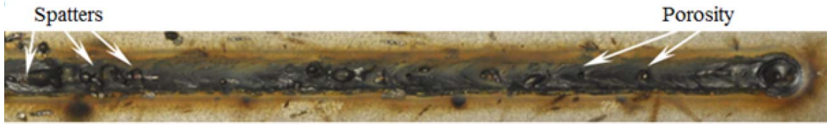
Laser welding of galvanized steel in a zero gap lap-joint that resulted in spatter and pore formation ( J Ma et al. 2012)
