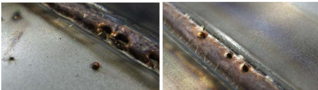
Examples of typical brazing defects porosity, spatter, bad wetting to the bottom sheet and bad wetting to the top sheet (Source J Wirth, EWM 2012)
