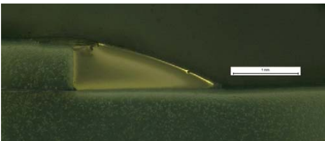
Good results with Plasmatron in straight a lap joint
