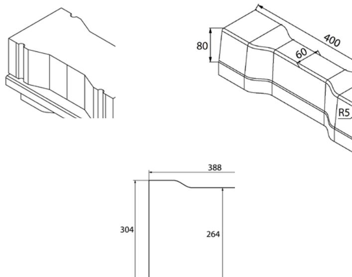
Figure 4: Geometry measurements of stamping tools and blank, all dimensions in millimetres.
