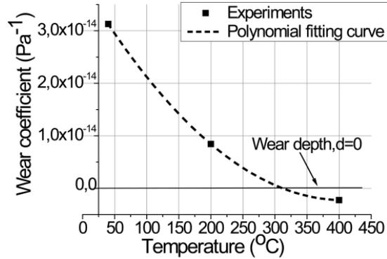
Figure 9: Wear coefficient used in the reciprocating wear model and wear rate
