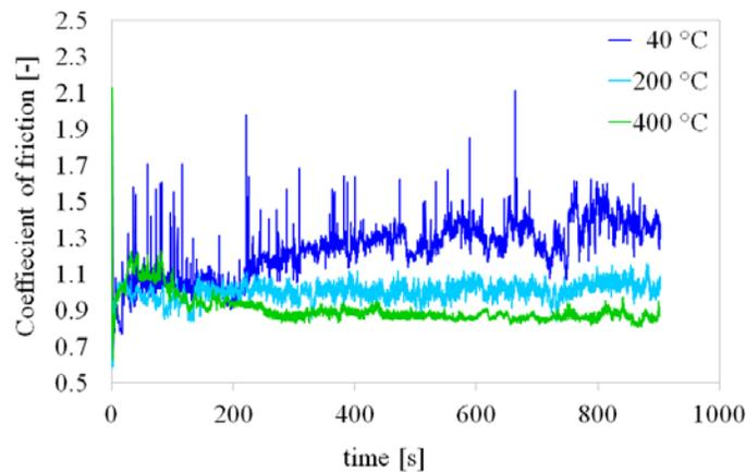
Figure 5: Coefficient of friction as a function of time at 40 °C, 200 °C and 400 °C as measured in the reciprocating experiments
