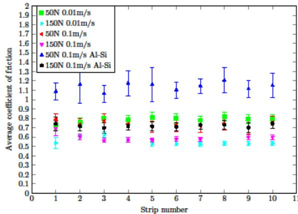
Figure 8: Average coefficient of friction of uncoated tool pins sliding against uncoated and Al-Si coated boron steel strips under different loads and sliding speeds
