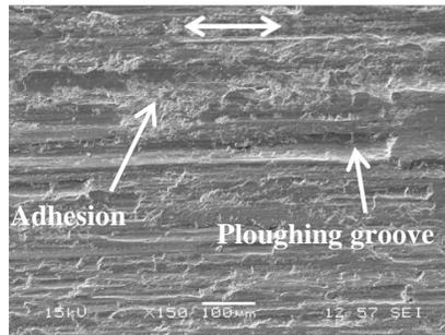
Figure 6: SEM image of the tool steel disc exposed to 40 °C; double arrow indicates sliding directions
