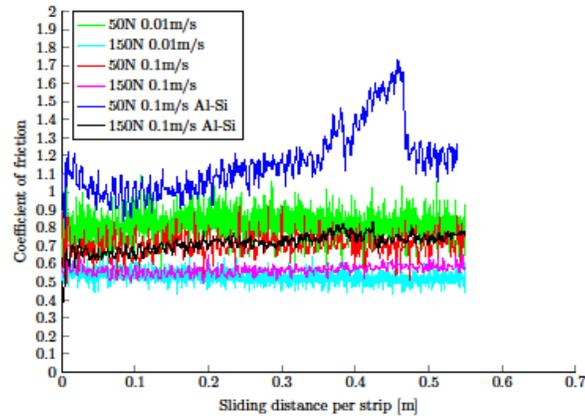
Figure 7: Coefficient of friction as a function of sliding distance for uncoated tools
