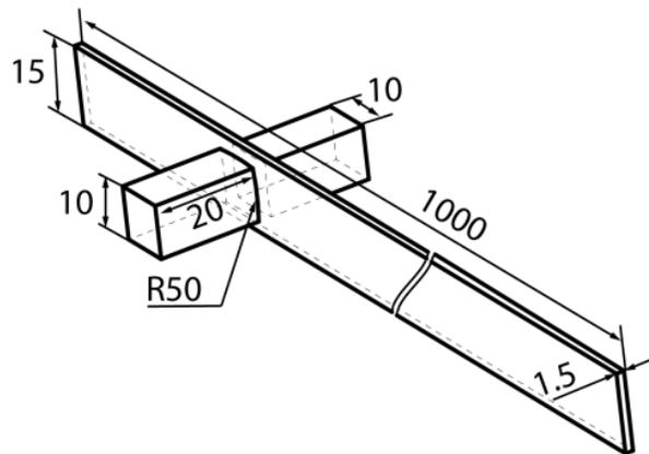
Figure 3: Configuration in the simulative tests; all dimensions are in millimetres
