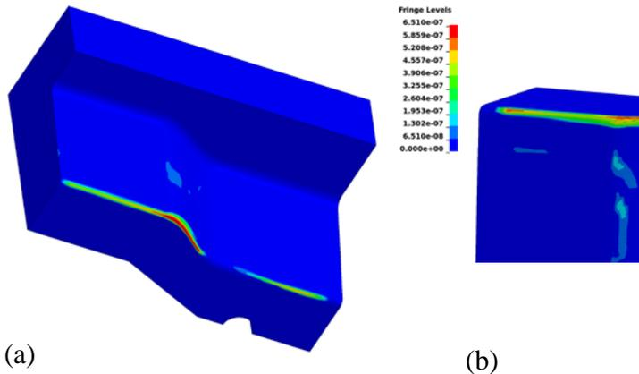
Figure 11: Distributions of wear depth in meters on stamping tool with the gap of 4.6mm after one stroke: (a) upper tool; (b) lower tool
