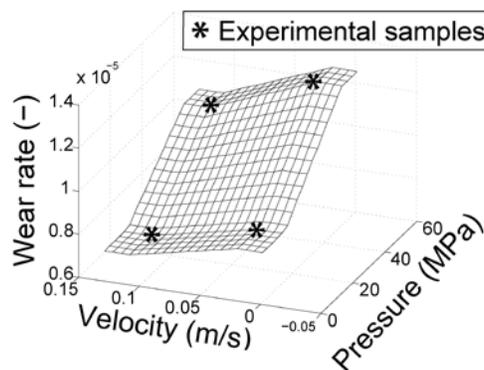
Figure 10: Wear rate used in the simulative wear model
