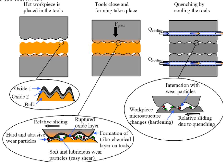
Figure 1: Schematic of thermomechanical forming process showing how tribological conditions change during one process cycle.
