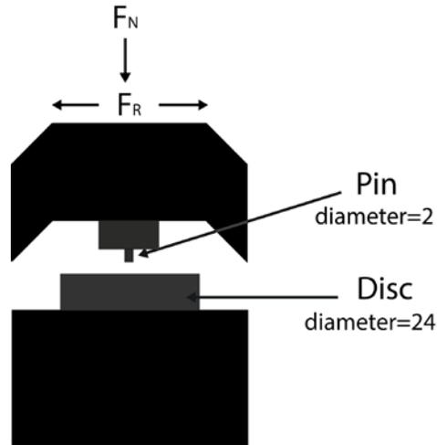
Figure 2: Configuration in the reciprocating test; all dimensions are in millimetres
