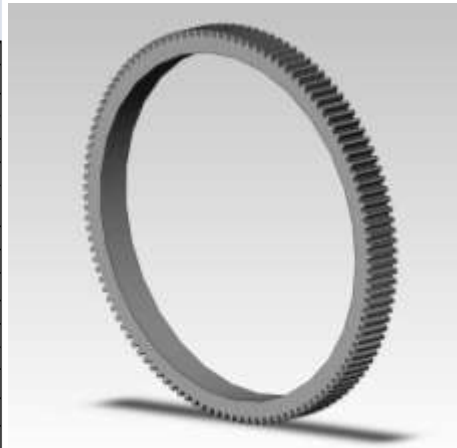
Fig 7. Geometry of ring gear for comparison of heat distortion at case hardening.
