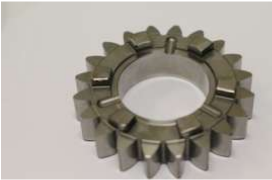
Fig 3. Gears in case hardened A85Mo5.
