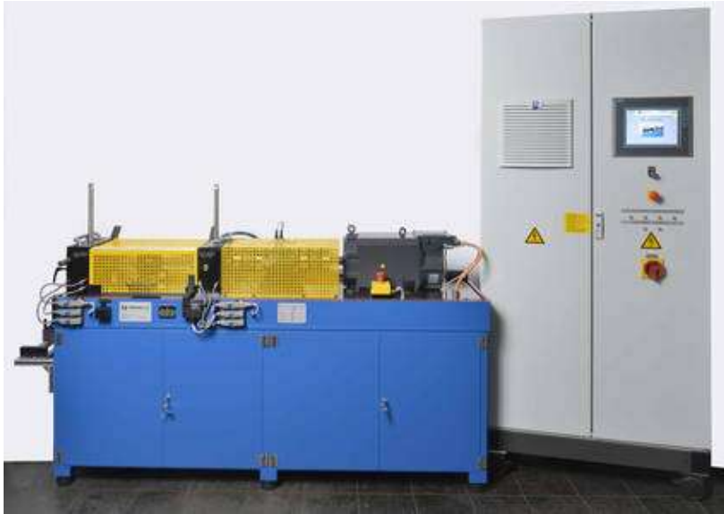
Fig 5. FZG-testrig for production of S/N-curves.
