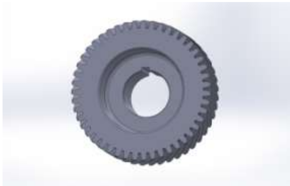
Figure 8. Conventional machined gear from forged steel.
