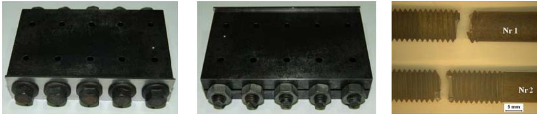
Fig. 3 Hydrogen embrittlement test by Japanese method. Assembly and failed screw.
