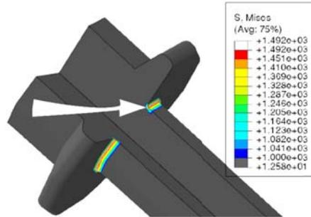
Fig. 4 Location of the initial plastic deformation in the fastener head region.
