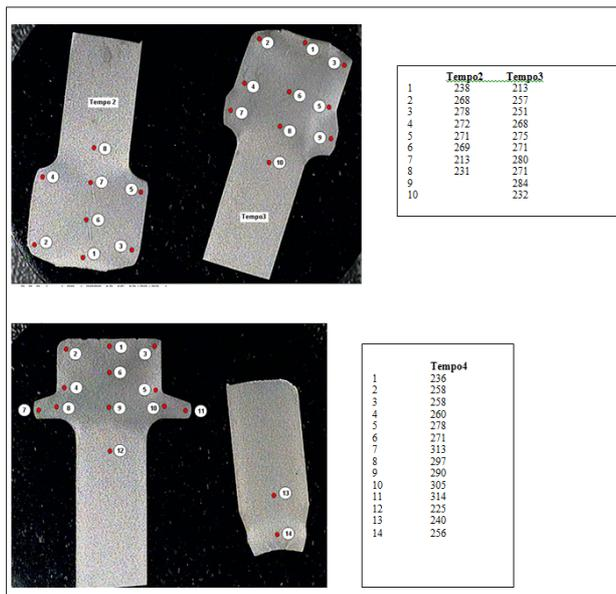
Fig. 6 Hardness measurements after cold forming steps 2-4.
