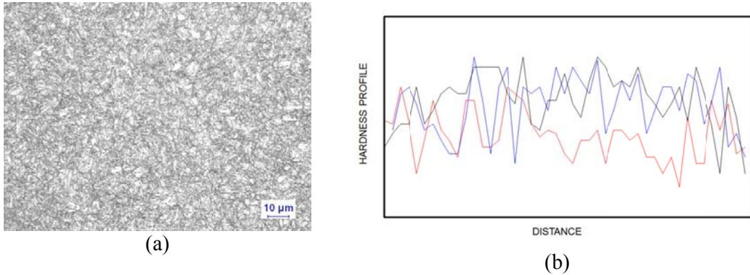
Fig. 7 (a) Fine grained and tempered martensite of B14 fastener. (b) Hardness profile.
