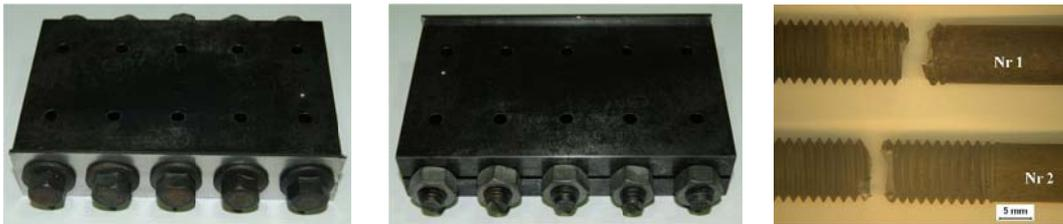
Fig. 3 Hydrogen embrittlement test by Japanese method. Assembly and failed bolt.
