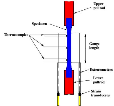
Fig. 2 Bofors creep test frame and assembly.
