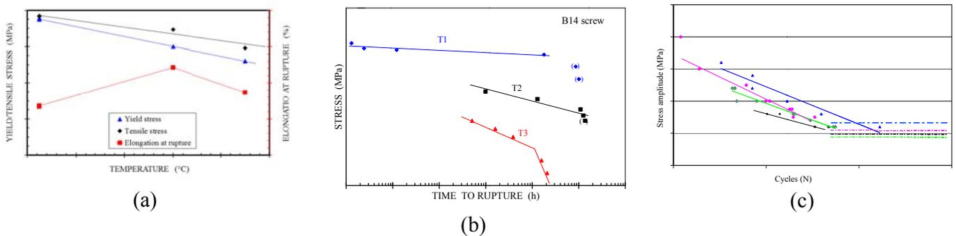
Fig. 8 Mechanical properties of B14 fastener. (a) Tensile properties. (b) Creep properties. (c) Fatigue properties.
