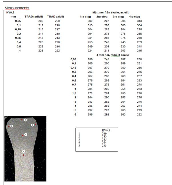
Fig. 5 Hardness measurements on wire.
