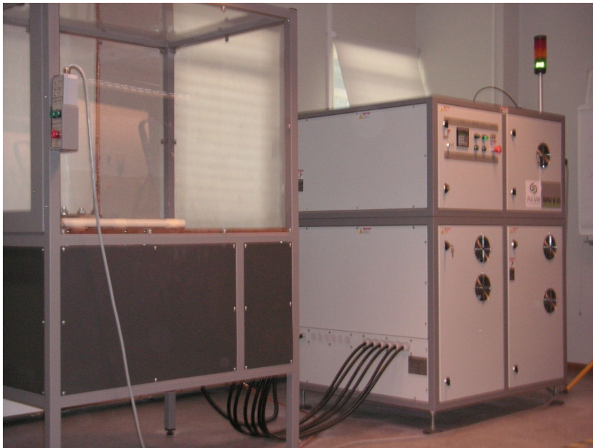
Figur 3 Magnetpulssystemet hos Swerea KIMAB
