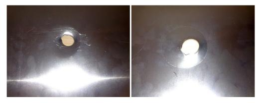
Figure 11 The results for the attempt to punch a hole in a Al sheet with magnetic pulse
