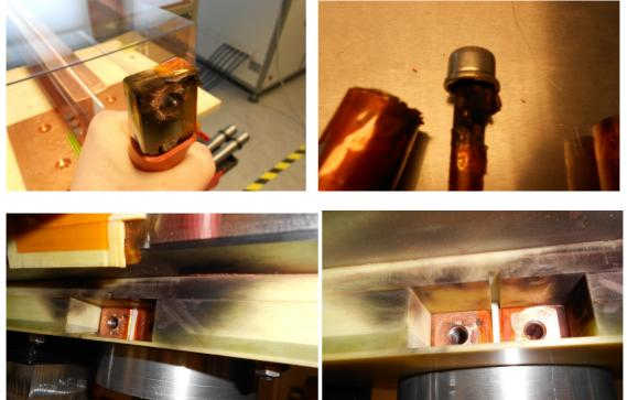
Figure 9 show spark erosion at the first trials of magnetic pressure punching tests.
