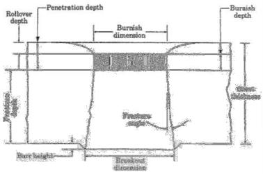
One interesting observation was that the fracture angle for the C20 steel was negative while for steel 1.4301 the angle was positive. The fracture angle is usually positive but this phenomenon can occur at high punching speed.
