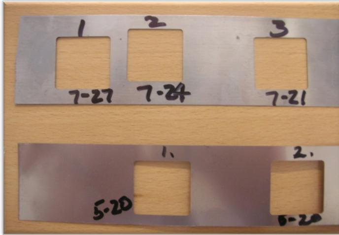
Figure 2 The high speed punched holes.
