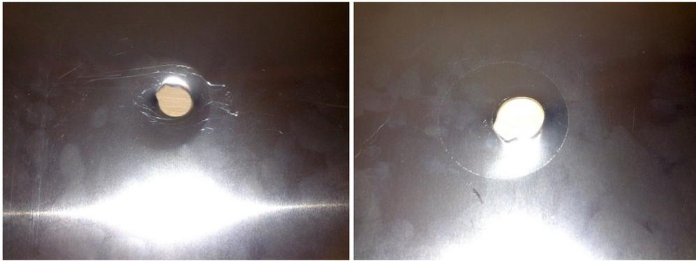
Figure 11 The results for the attempt to punch a hole in a Al sheet with magnetic pulse
