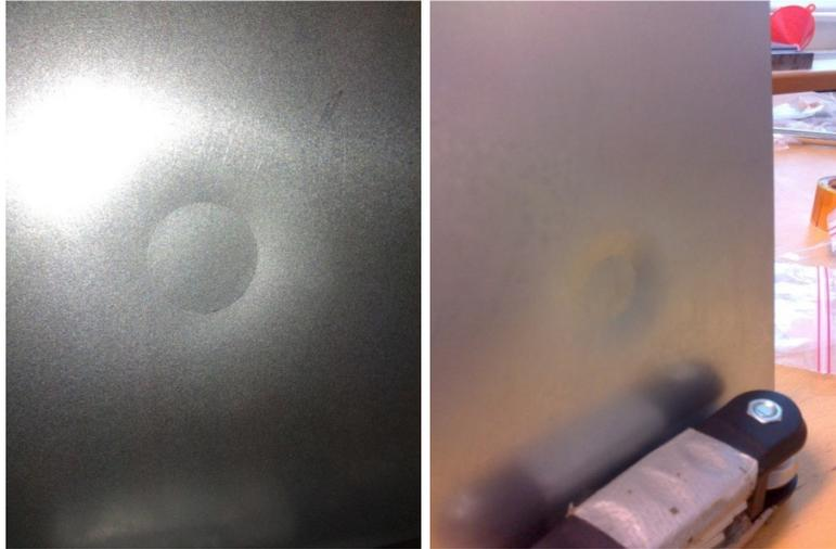
Figure 10 The results for the attempt to punch a hole in a steel sheet with magnetic pulse
