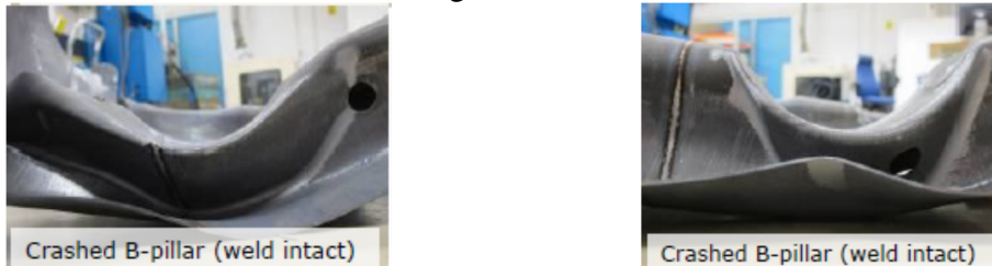
Figure 15 – Crash-tested B-pillars (with AlSi-coating). The laser-hybrid welds are intact. Left image: test No 13; Right image: test No 5. Both were welded without patches.
