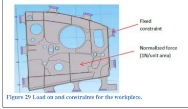
In Comsol 4.2a (FEA) the eigen frequency study reveals the natural modes of vibrations at which the structure shows resonances if excited. Similarly in Test Lab rev 11a (EMA) the natural vibration modes are selected by viewing FRF and indicating the stable regions which shows concentration of chatter amplitude.
