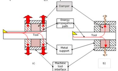
Figure 32 Energy propagation paths. (a) Bypass through metal-to-metal contact. (b) No bypass, energy flows through damping material.
