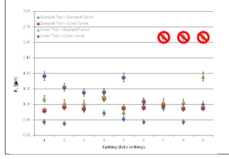
Figure 35 Machining test results, surface roughness. Comparison between the conventional tool clamped in conventional turret and in the damped turret, as well as the damped tool clamped in the conventional turret and in the damped one. The conventional tool clamped in the conventional turret could not perform at setting 7, 8 and 9 due to excessive instability.
