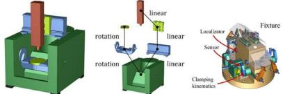
Figure 3 ISO 10303 STEP kinematics augmented with terminology.
