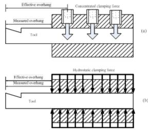
Figure 31 Comparison between conventional screw clamp (a) and hydrostatic clamp (b).
