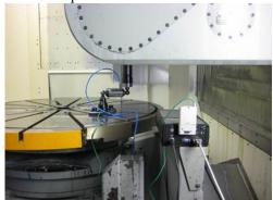
Figure 15 The loaded double ball bar system (LDBB). The LDBB is a result of a collaborative development by the two Swedish companies Scania CV AB and CE Johansson AB and KTH Royal Institute of Technology.
