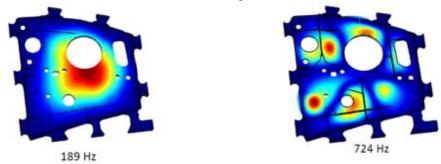
Figure 30Simulation of modes of vibration.
