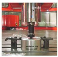
Figure 17 Contactless excitation and response system (CERS). The actuator hardware with on-board displacement sensors is clamped on the machine tool table. The specially developed cutting tool is inserted in actuator unit. The contactless excitation is done with inductive coils and the response measurements are done via displacement sensors placed 90° apart.
