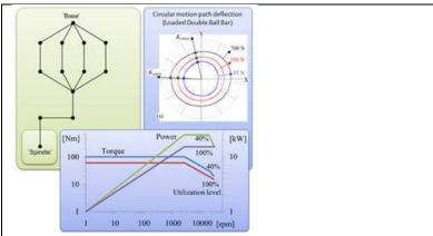
Figure 4 Kinematic structure as context for loaded double ball bar (LDBB) result and spindle motor properties.
