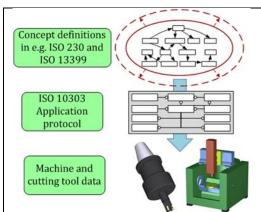
Figure 6 Modeling approach combining extendable terminology with STEP data model.
