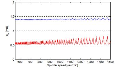
Figure 34 Stability limit diagram for conventional tool (red) and HDI-tool (blue).
