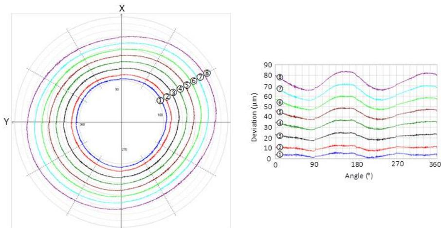
Figure 16 Deflection diagrams in X-Y plane. Deflection diagram as function of applied load  $P_{force}(1-8) = \{36; 112;$
