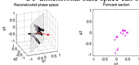
**Figure 23** 3-dimensional state space with a flat Poincaré plane (left) and the corresponding 2-dimensional Poincaré section (right).
