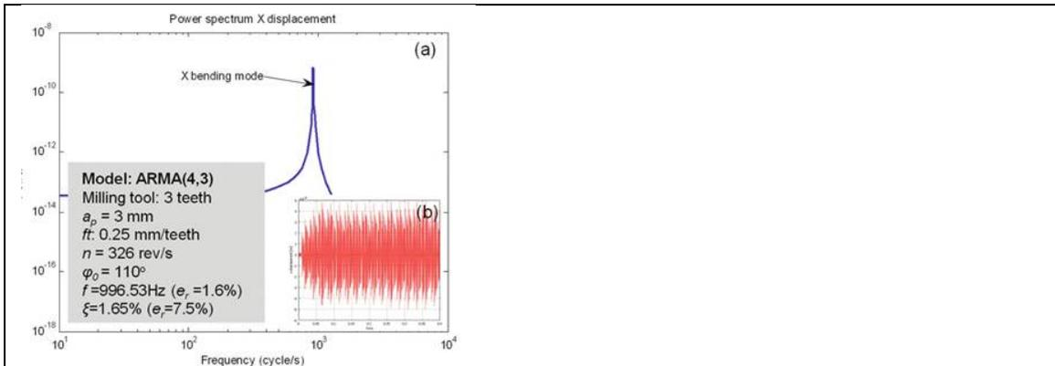
**Figure 8 Power spectrum of a ARMA (4, 3) at tooth passing frequency close to 980 Hz. (b) time domain stable vibration in X direction.**
