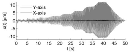
**Figure 21** Calculated vibration amplitudes. Increasing the table speed of 50 rpm every 5 seconds.
