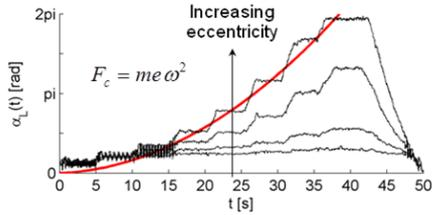
**Figure 20** Measured angle in Lissajous figure with increasing eccentricity of the unbalanced weight. Increasing the table speed of 50 rpm every 5 seconds.
