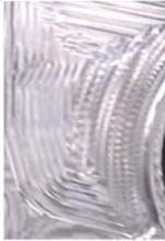
Figure 26 Poor surface finish after machining.
