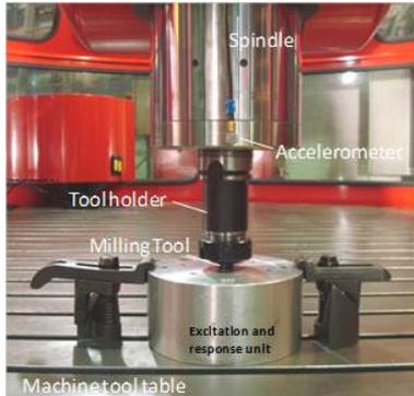
**Figure 17** Contactless excitation and response system (CERS). The actuator hardware with on-board displacement sensors is clamped on the machine tool table. The specially developed cutting tool is inserted in actuator unit. The contactless excitation is done with inductive coils and the response measurements are done via displacement sensors placed 90° apart.
