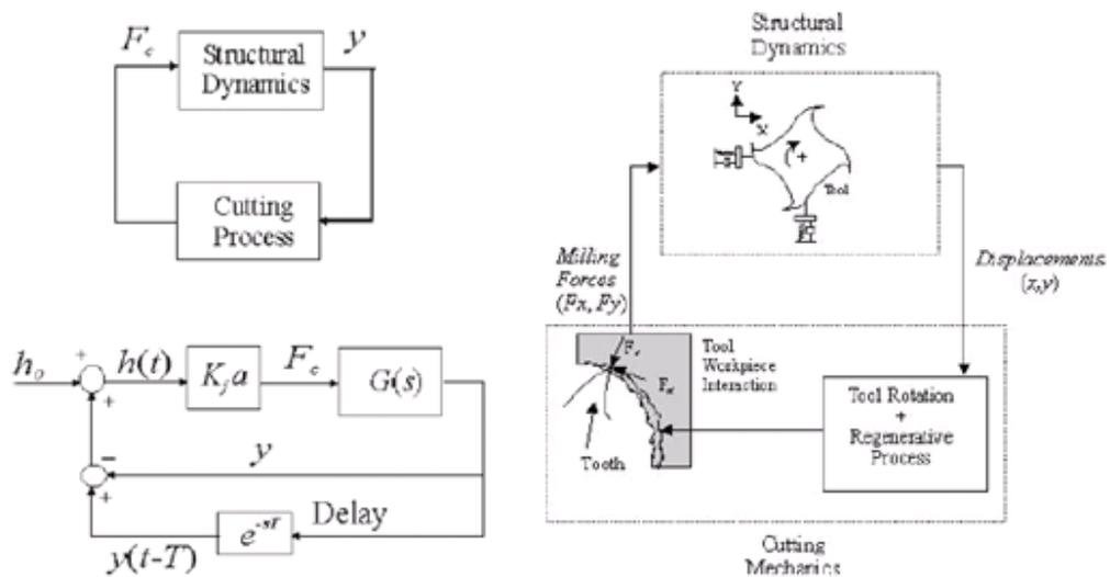
Figure 27 Dynamics of orthogonal milling operation.
