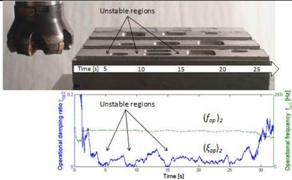
Figure 14 RARMA identification of ODP in face milling. Top, the experimental setup in which the workpiece is prepared with holes and pockets to replicate time-varying cutting condition, and bottom, tracking the variation of the second identified ODR and frequency.
