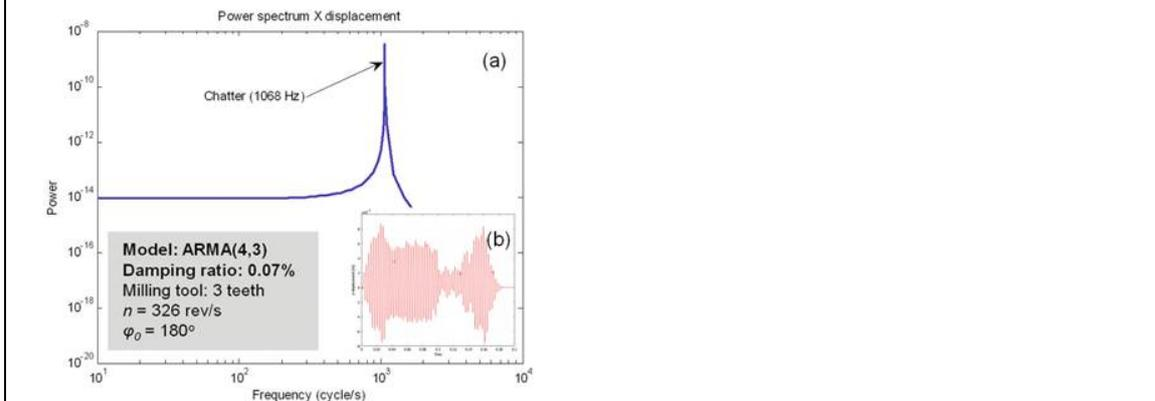
**Figure 9 Parametric identification: power spectrum for unstable machining system, (b) time domain chatter as a regenerative phenomenon between consecutive teeth, vibration in X direction. The nonlinear effect due to the loss of contact between tool and work is apparent.**
