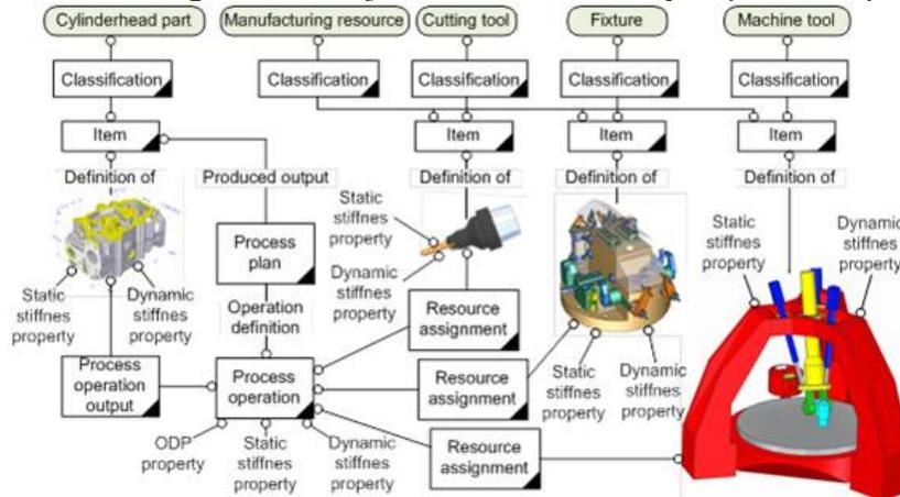
Figure 7 Coherent industrial data based on ISO 10303.
