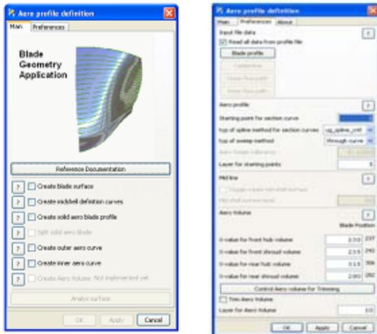
Figure 10 User interface of aero-blade application.
