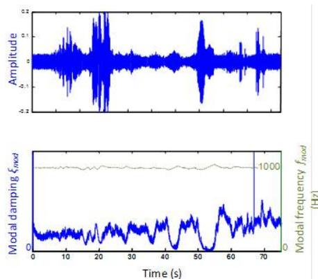
**Figure 18** Damping ratio and natural frequency. RARMA-modal estimation on accelerometer signal in Y direction. Contactless random excitation.
