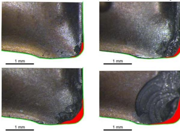
Figure 24 Different levels of tool wear.
