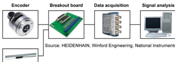
**Figure 19 Measurement chain from the encoder output to the measurement computer.**
