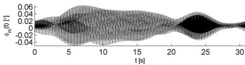
**Figure 22** Torsional oscillations in the time domain for 5-toothed milling based on measurement of the encoder signals.
