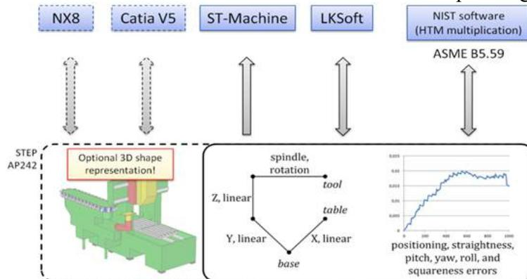
Figure 5 System integration via data consolidation.
