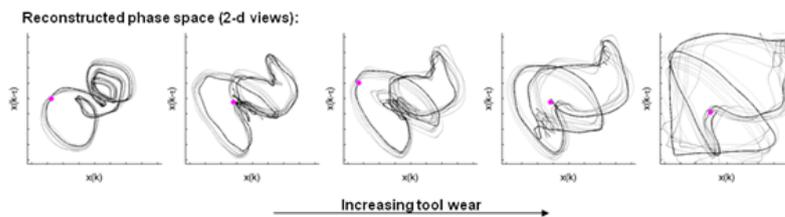
Figure 25 2-dimensional images from the state space at different levels of tool wear.
