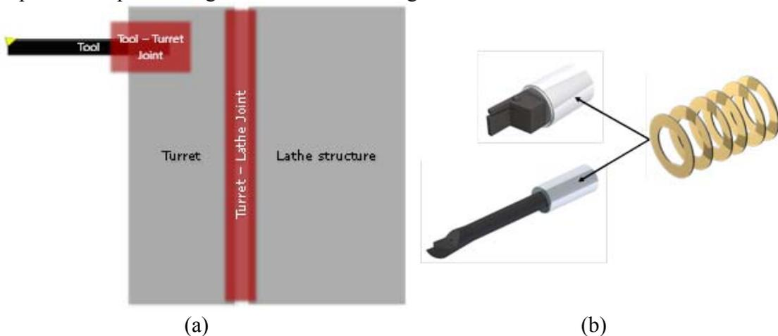
Figure 33 (a) Joints treated in the CNC-turning centre. (b) Multiple layers of VE polymer metal composite plates implemented in the parting-off tool and in the boring bar.
