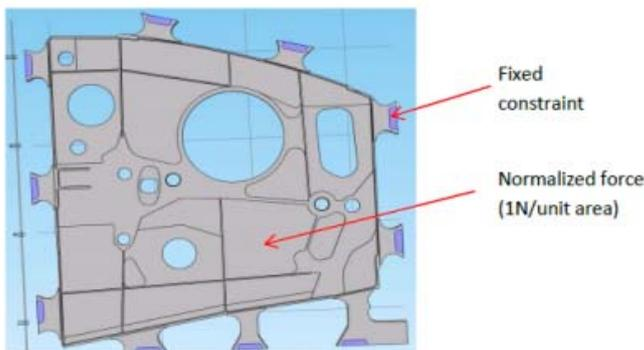
Figure 29 Load on and constraints for the workpiece.
