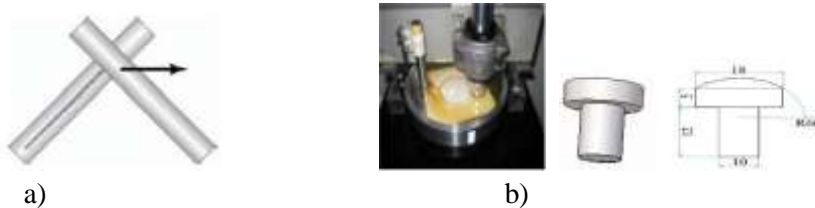
Figure 2 Wear testing equipment used: a) Tribological load scanner b) Pin-on-disc
